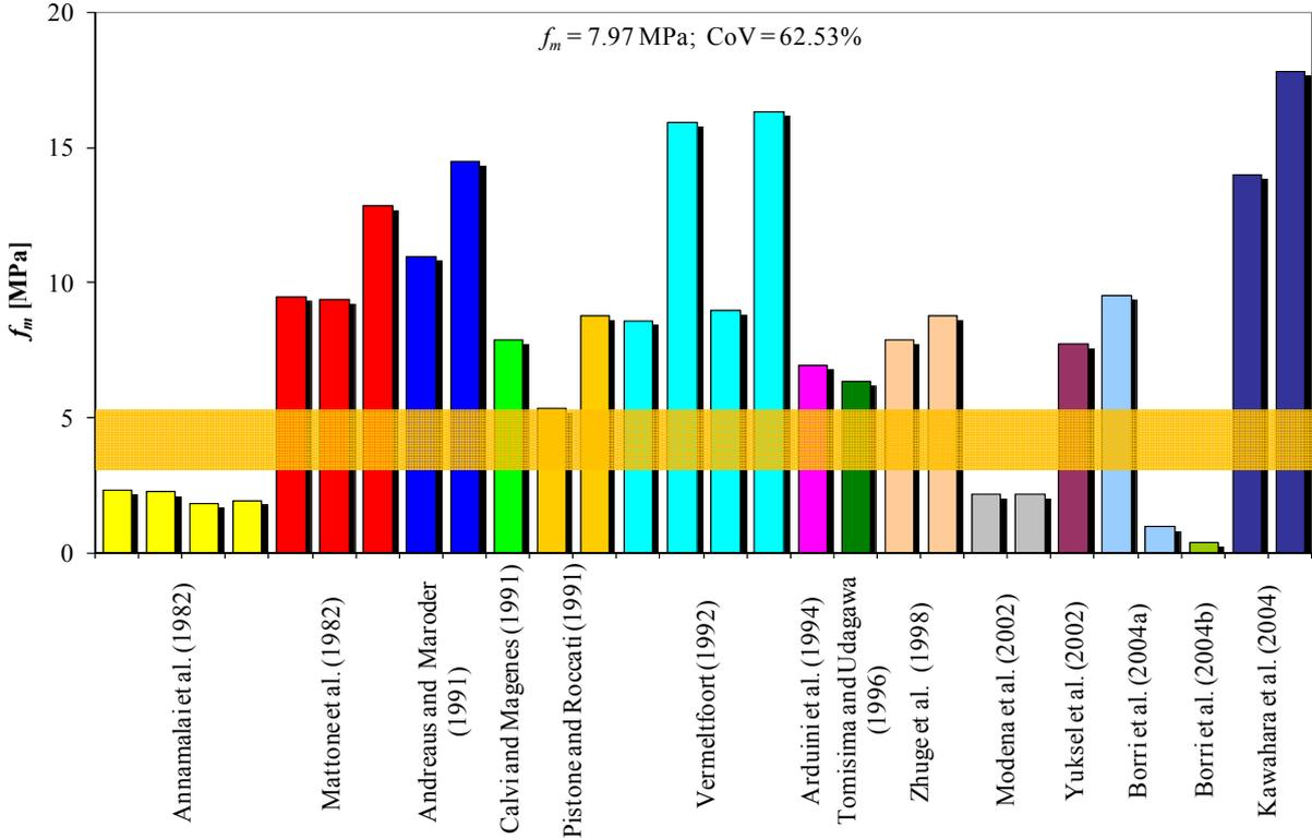
Figure 1. Experimental data on uniaxial compressive strength of brick masonry class 1
