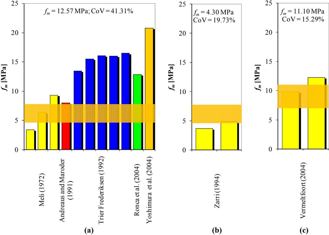
Figure 2. Experimental data on uniaxial compressive strength of brick masonry classes (a) 2, (b) 3 and (c) 4
