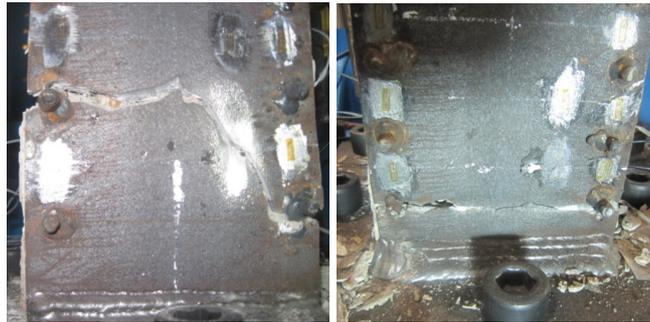
**Figure 8.** Low-cycle fatigue fracture in Specimens PE2 (left) and PE3 (right)
