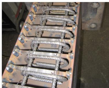
**Figure 5.** Specimen with additional buckling-delaying plates
