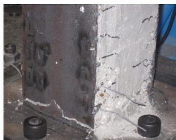
**Figure 10.** Low cycle fatigue fracture in Specimen PE7
