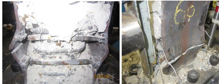
**Figure 9.** Low cycle fatigue fracture in Specimen PE4: link fracture (left) flange-through fracture (right)
