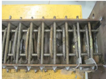
**Figure 4.** Specimen with additional buckling-delaying bars
