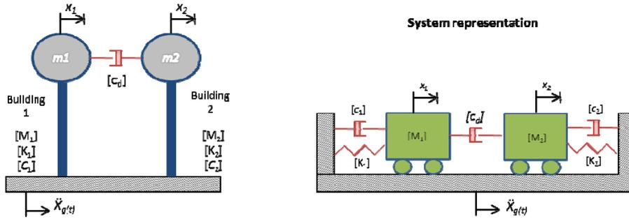
**Figure 3.** Single degree of freedom masses coupled.
