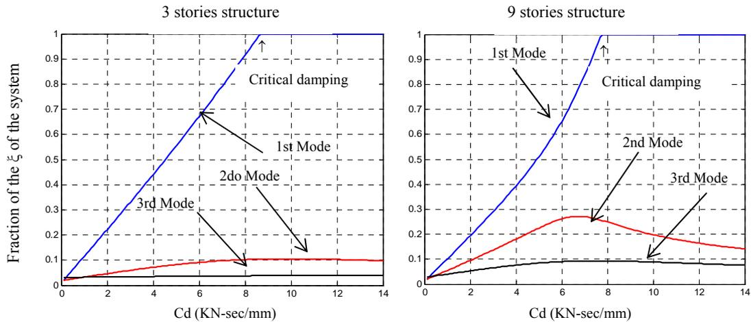
**Figure 8.** Variation of the critical damping of the system.
