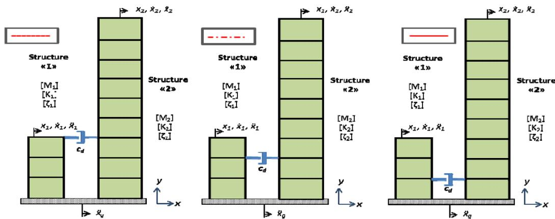
Figure 10. Models used to determine the best position of the damper.
