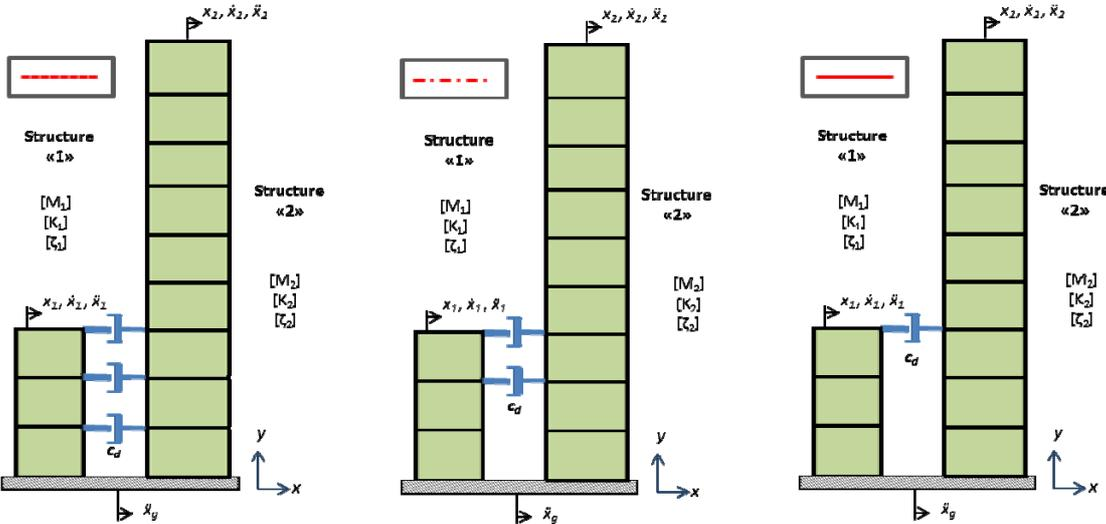
**Figure 12.** Models used to determine optimal position of the damper.
