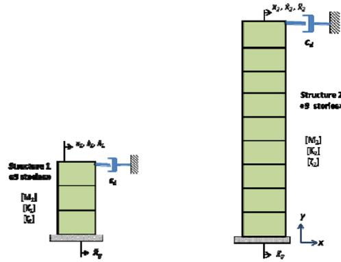
**Figure 7.** Position of a fixed damper on each of the SAC structures.
