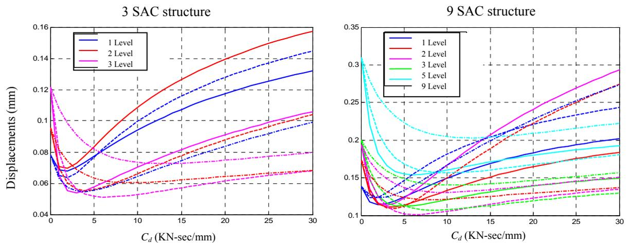
Figure 11. RMS displacement responses for the different positions of the dampers.
