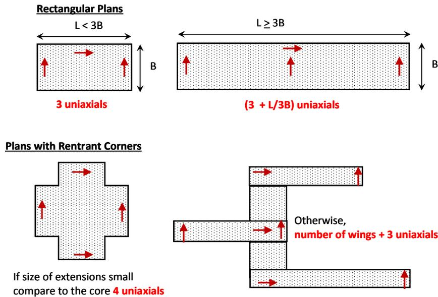
**Figure 3.4.** Accelerometer distribution over the plan
