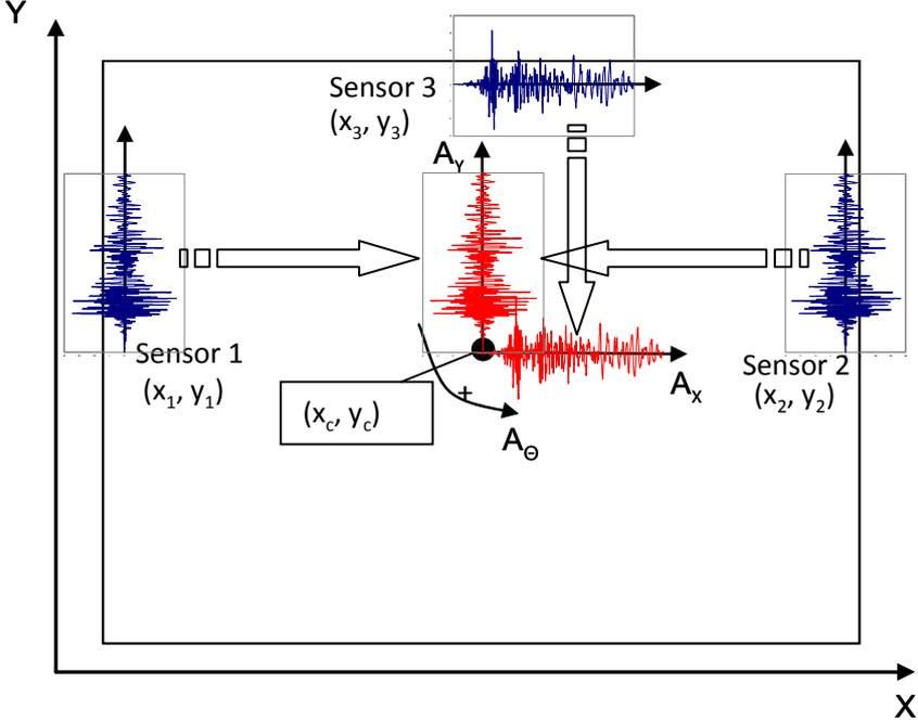
**Figure 3.2.** Typical sensor layout on a rigid diaphragm rectangular floor
