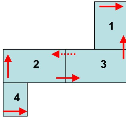
**Figure 3.3.** Complicated floor layouts may be divided in simpler zones for establishing an efficient sensor layout
