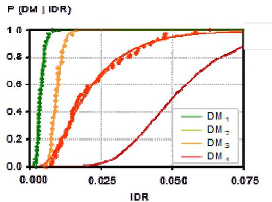
**Figure 2.1.** Fragility functions relate probability of damage severity to a measured demand parameter such as interstory drift ratio (Miranda 2006)
