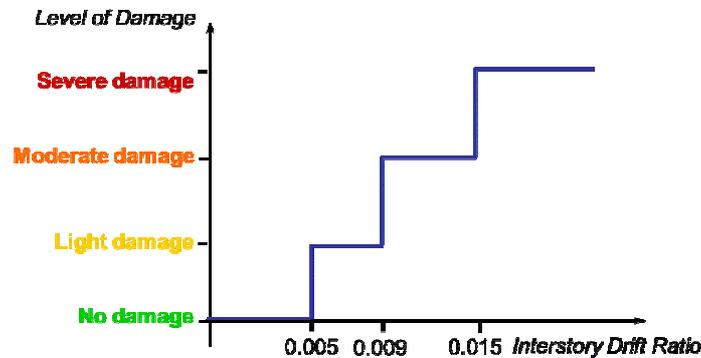
**Figure 2.2.** Unrealistic view of damage as a step function implied by building codes, and deterministic guidelines and standards (Miranda 2006)
