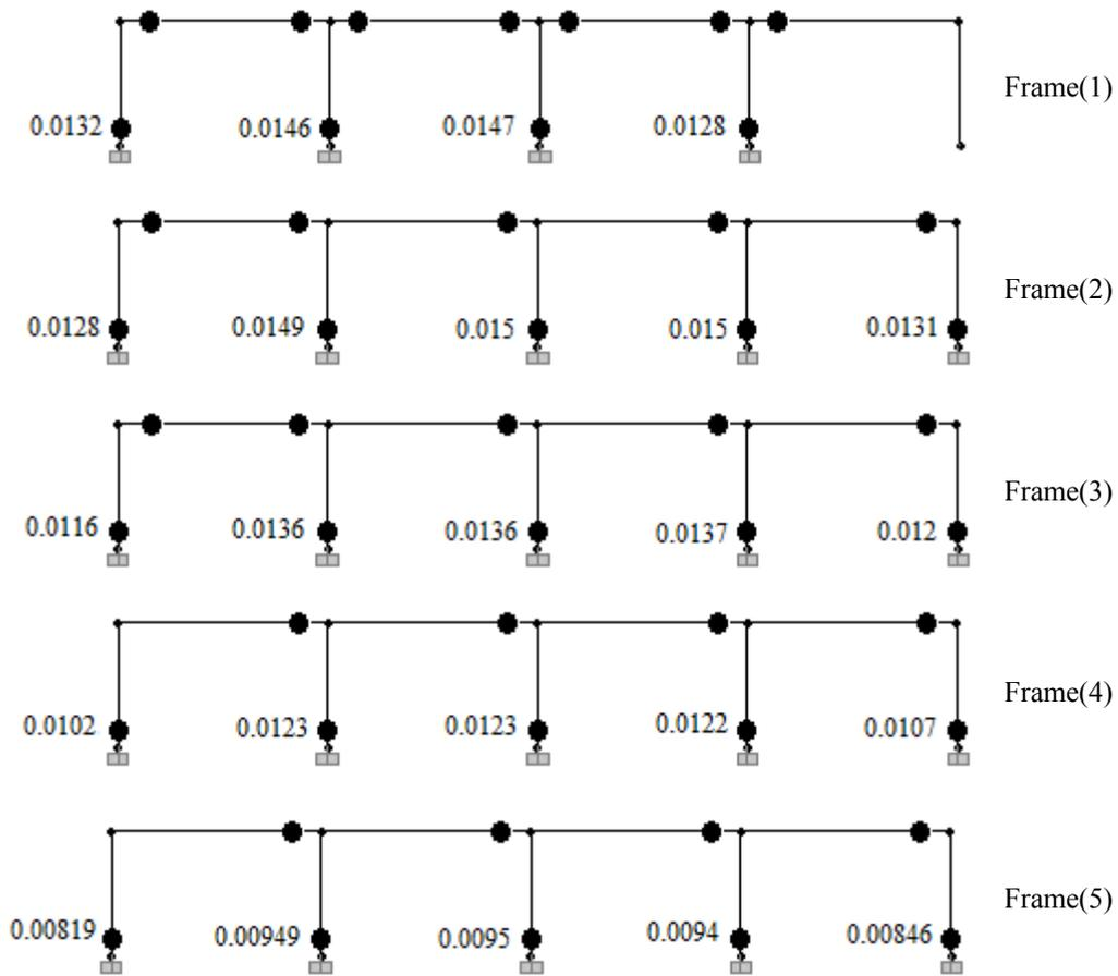
**Figure 3.5.** Rotation of the plastic hinges of the damaged building at the displacement of 6.4cm
