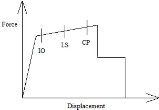
Figure 3.2. Behavior of the plastic hinges of the beams
