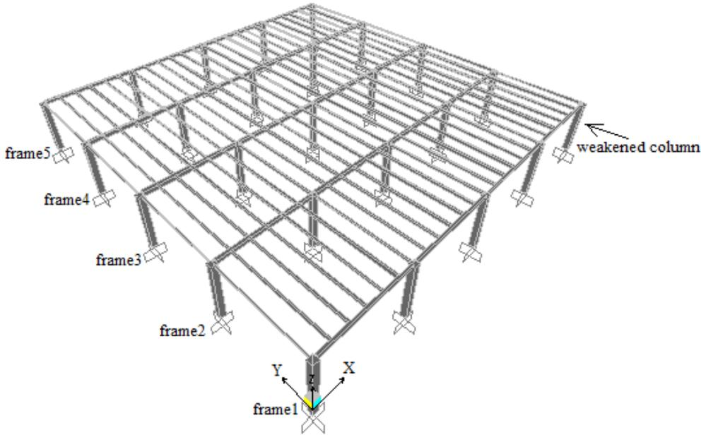
Figure 3.3. Three-dimensional finite element model of the second building
