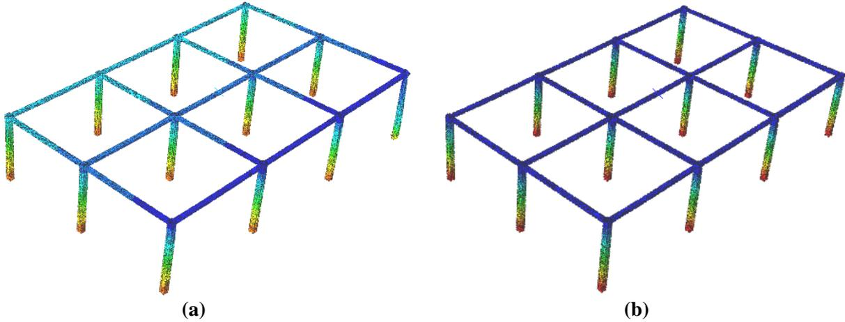
Figure 3.1. Deformation of the (a): damaged and (b): primary structures subjected to lateral loading
