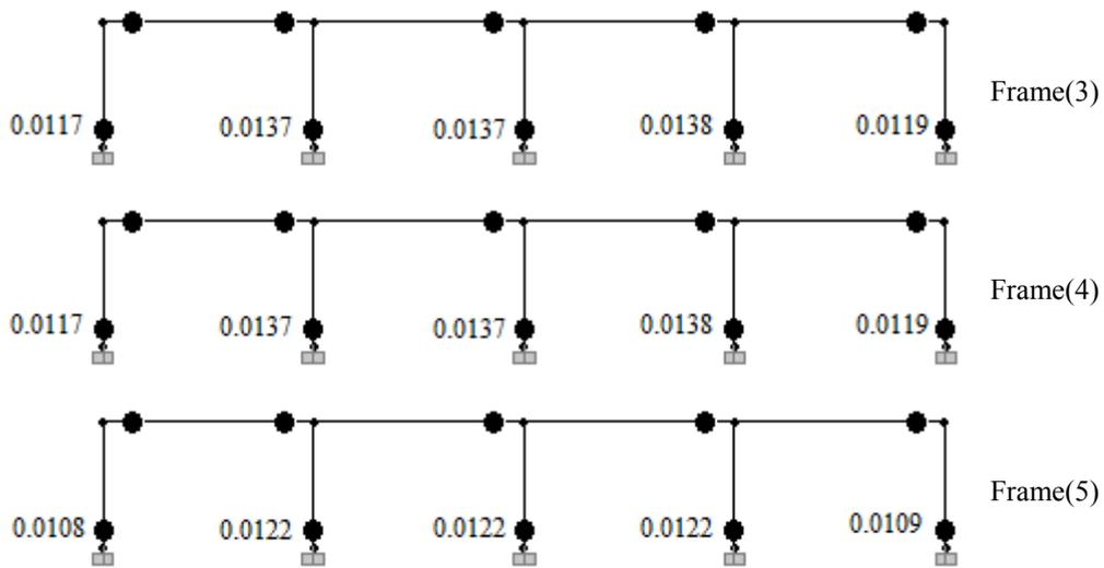
**Figure 3.4.** Rotation of the plastic hinges of the primary building at the displacement of 6.4cm
