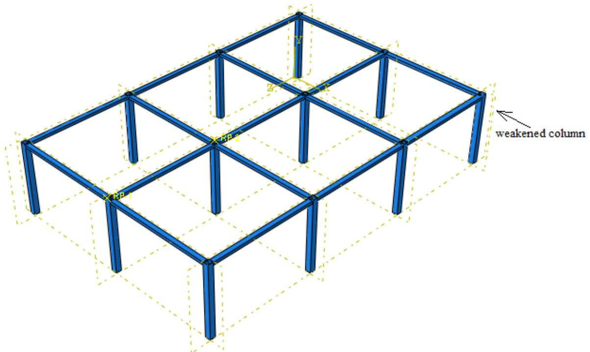
**Figure 2.1.** Three-dimensional finite element model of the first building
