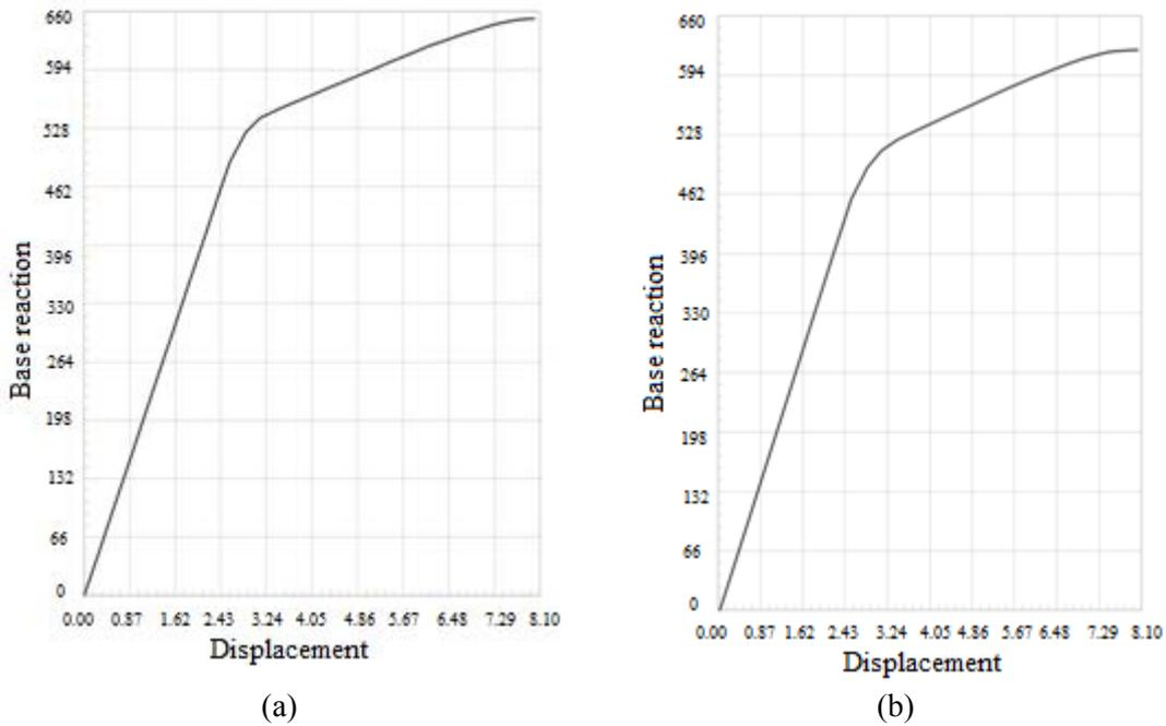
**Figure 3.8.** Push-over curve of (a): primary and (b): damaged one
