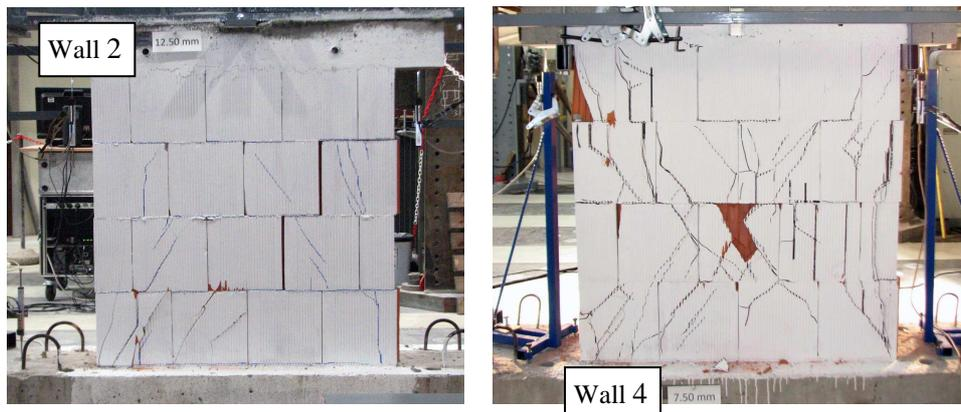
**Figure 6.** Collapse of wall 2 (left) and wall 4 (right)
