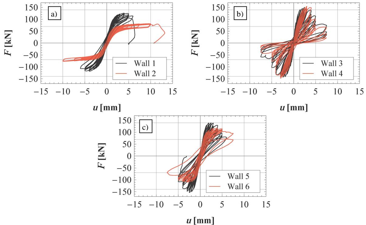
**Figure 4.** The effect of the level of precompression for a) cantilever, b) fixed rotations and vertical displacements and c) fixed rotations and vertical load. Hysteretic response of walls at 20 % precompression is drawn in black, of walls at 10 % in red
