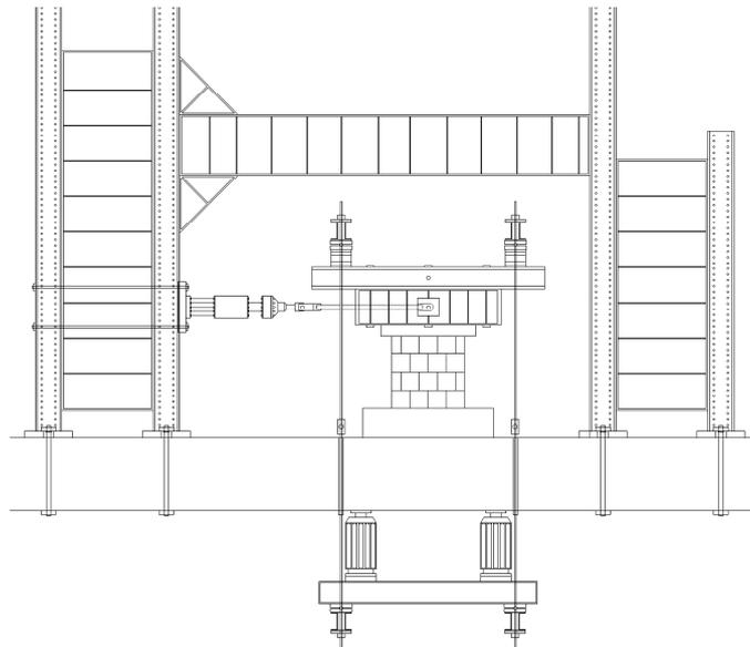
**Figure 3.** Test setup and test walls
