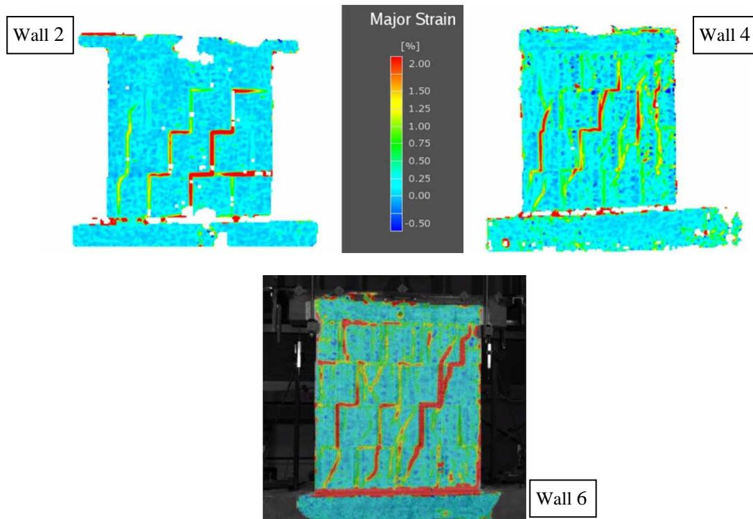
**Figure 7.** Major strain fields for walls 2 (top left), 4 (top right), and 6 (bottom center)
