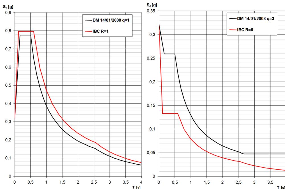
**Figure 2.2.** Elastic and design spectra comparison between DM 14/01/2008 and IBC
