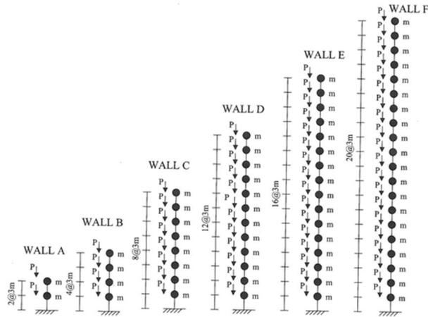
**Figure 3.1.** Cantilever walls investigated into the analysis [Priestly et al.]
