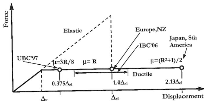
Figure 4.2. Estimates of Design Displacement from Different Force-Based Codes for R=4 [Priestly et al.]
