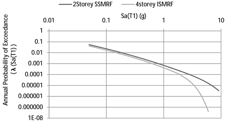
Figure 3. Hazard curves for the case study frames.
