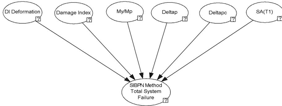
**Figure 4.** The developed BPN for the 1-bay, 2-storey SSMRF using GeNIe software.
