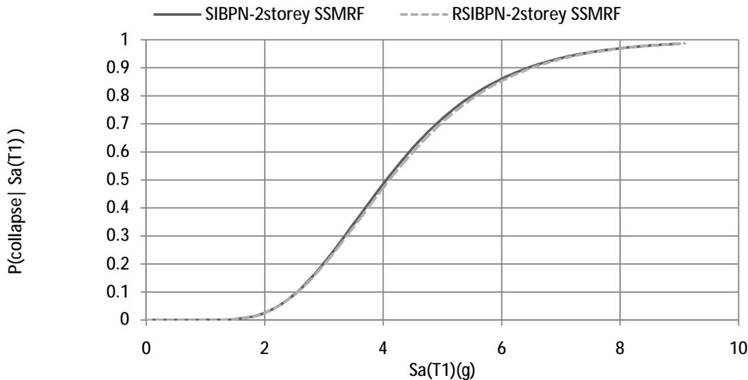
Figure 7. Fragility Curves for the case study SSMRF using SIBPN and RSIBPN approaches
