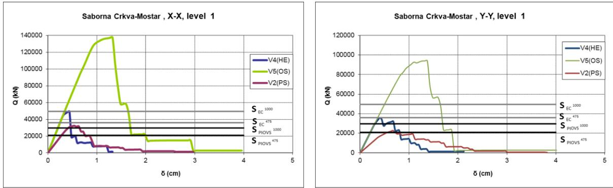
Figure 4.4. Comparative presentation of bearing capacity, level 1
