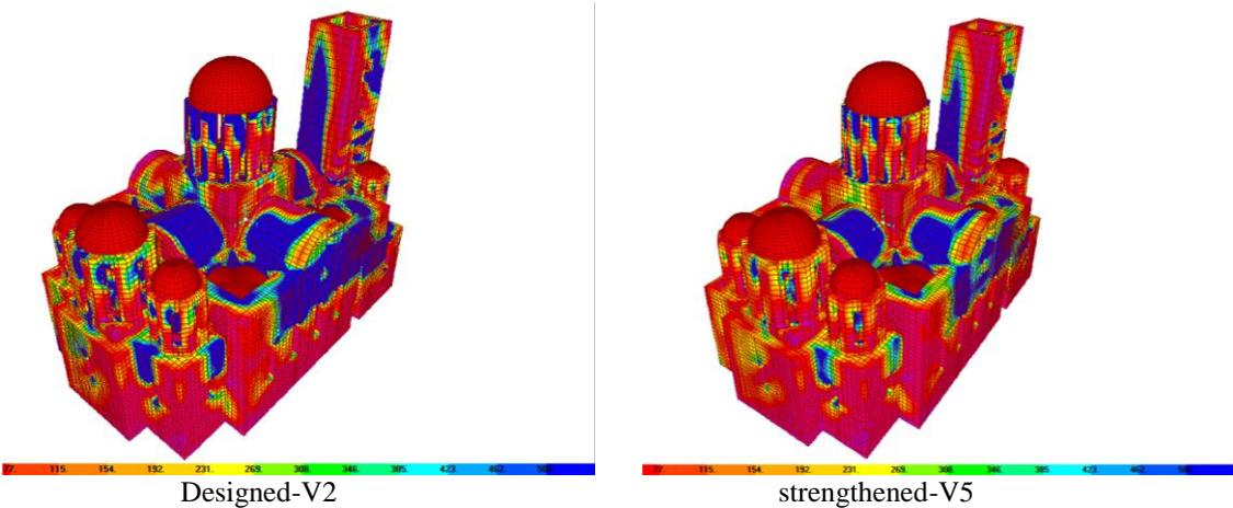
**Figure 4.7.** Main tensile stresses (dead weight +  $S_y^{EuroCode}$ )
