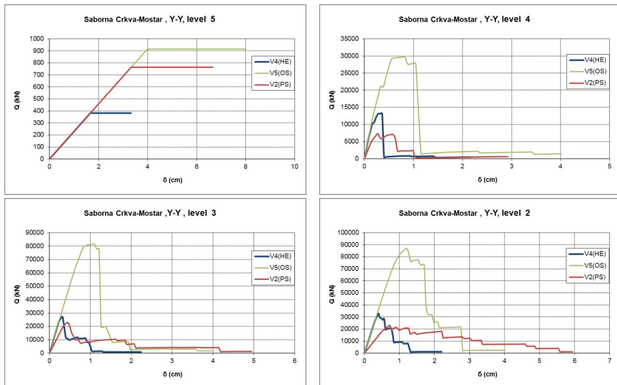
Figure 4.3. Comparative presentation of bearing capacity, transverse direction, (level 2-5)
