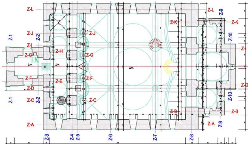
**Figure 4.1.** Ground floor plan of the designed church structure
