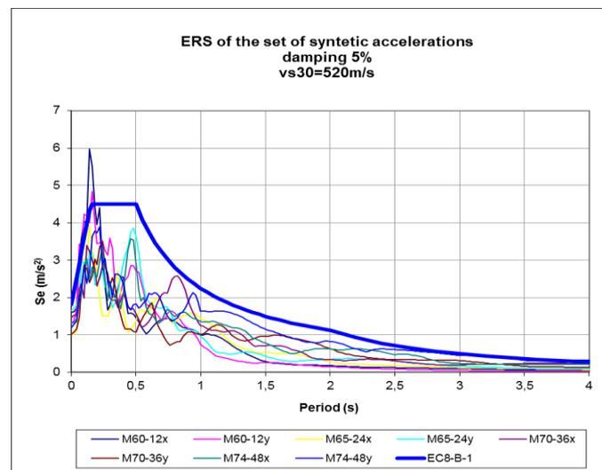
**Figure 3.1.** Elastic response spectrum of the set of synthetic accelerations
