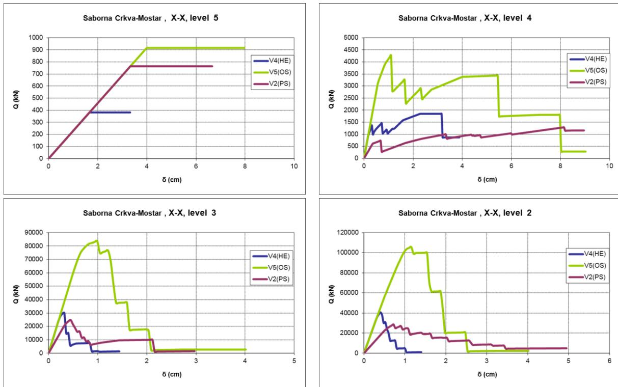
Figure 4.2. Comparative presentation of bearing capacity, longitudinal direction (level 2-5)
