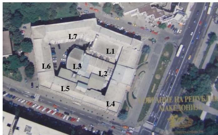
**Figure 3.1.** Individual structural units of the building (Units L1 – L7)
