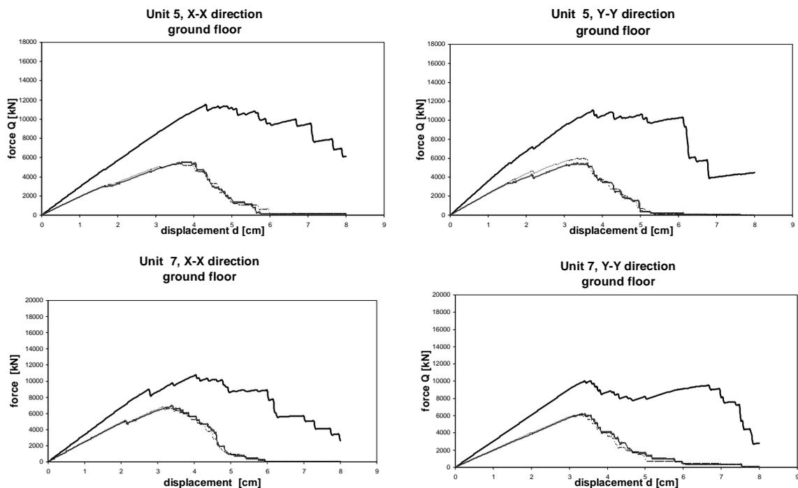
**Figure 4.2.** Comparative Q-d diagrams for characteristic units
