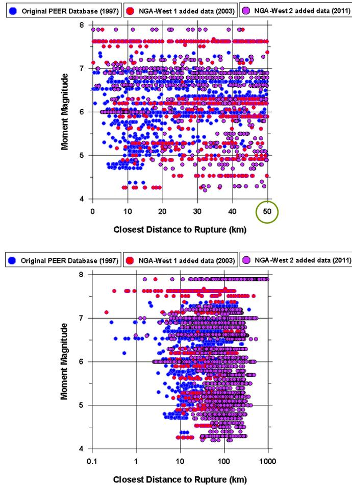
**Figure 1.1.** Magnitude-distance distribution of earthquakes in the NGA-West2 moderate-to-large magnitude database for near-source distances (top) and all distances (bottom)
