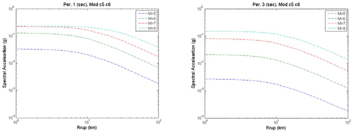
**Figure 2.1.** New near-source magnitude saturation term showing total (left) and partial (right) saturation
