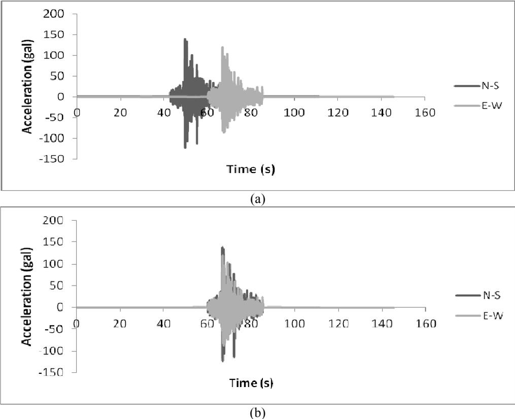
**Figure 3.** (a) Waveform of the processed recording showing the time lag due to separate zero pads in horizontal components and (b) Waveform of the same recording after shifting to align the start times (Record name: 19990817000139\_1404)
