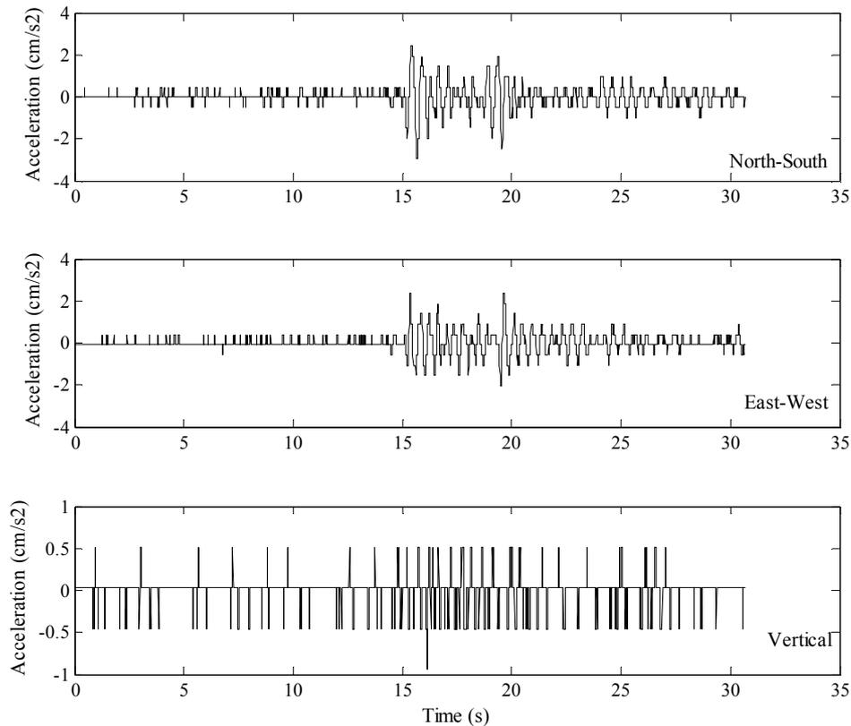
**Figure 2.** A sample record with (NS, EW and Vertical components) that was discarded due to low digitizer resolution (record name: 19981008204912\_2401).
