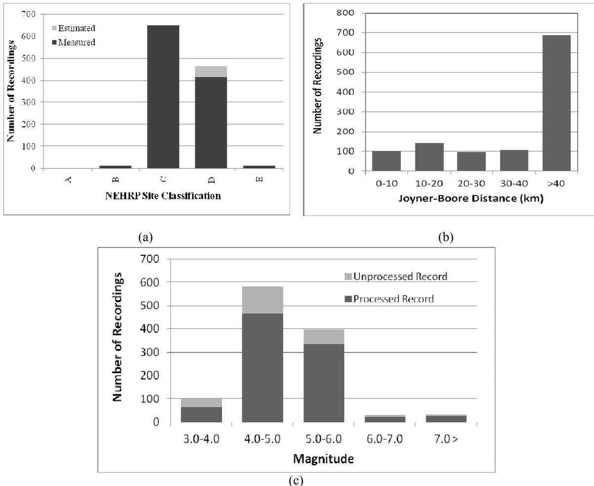
**Figure 1.** Distribution of the recordings in the comparison dataset with respect to (a) NEHRP site classification, (b) Joyner-Boore distance, and (c) magnitude.
