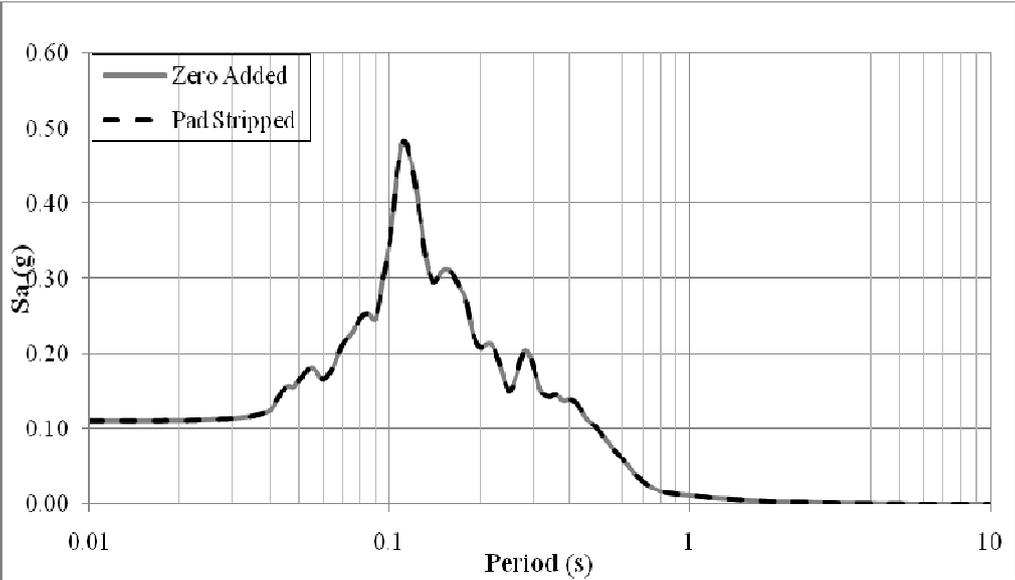
**Figure 4.** GMRot150 horizontal spectra for the same recording with zero pads cut-off (denoted by pad-stripped) from the long component and zero added to the short component for alignment (denoted by zero-added) (Record name: 19991107165434\_9906)
