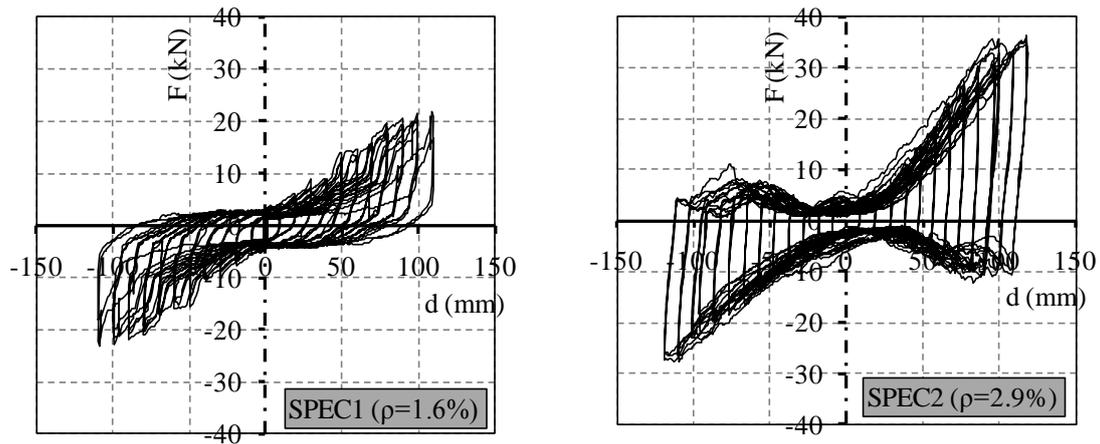
**Figure 3.3.** Hysteresis loops for the two specimens representing an 1:2 scale pair of walls
