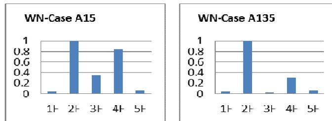
**Figure 2.** Stress Index under Full Observation (Multiple Stories Damaged, Input: White Noise)
