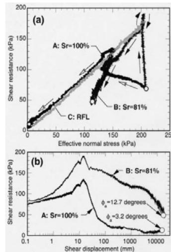
**Figure 10.** Shear versus Normal Stress and Shear Resistance versus Shear Displacement Relations Obtained from Undrained Ring Shear Tests (Konagai et al. 2002)
