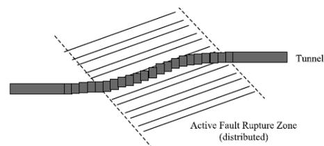
**Figure 2.** Articulated Tunnel Design to Distribute Shear Deformation across Fault Rupture (Russo et al. 2002)
