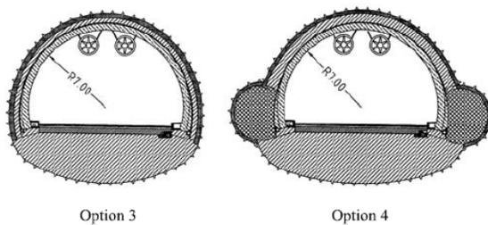
**Figure 3.** Segment Options of Tunnel Cross Section (Amberg and Russo 2001)
