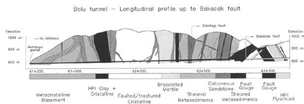
**Figure 1.** Zekidagi and Bakacak Active Faults Along Tunnel Profile (Russo et al. 2002)
