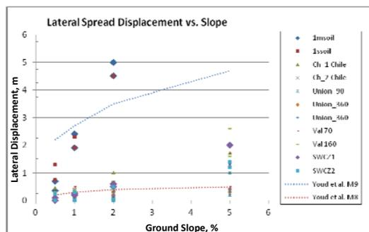
Figure 14. Results from FLAC deformation analyses as compared with those by Youd et al. (2002) method.
