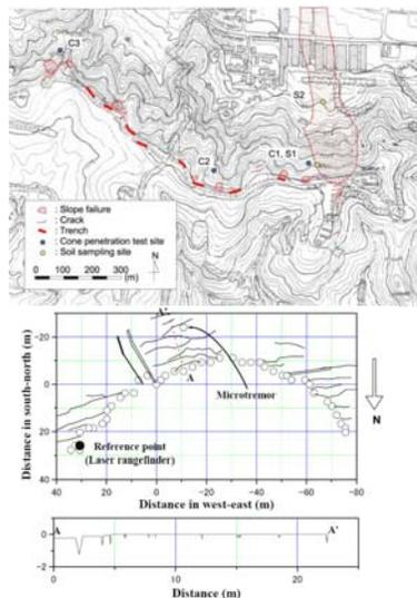
**Figure 9.** Topography in the Vicinity of the Las Colinas Slide and Crack Pattern along Top Edge of the Slide (Konagai et al. 2002)
