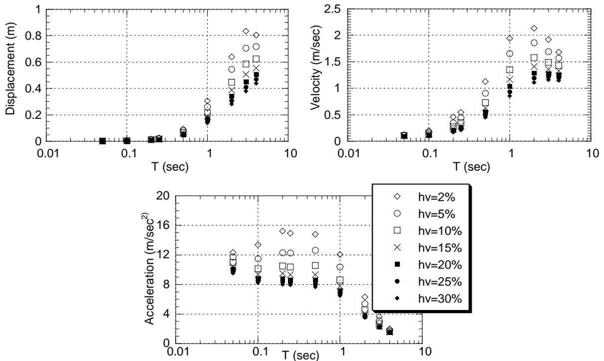
Fig.2.1.2 Seismic responses of simplified NPP model
