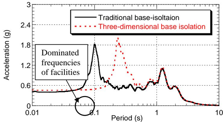
Fig.1 Floor response spectrum of two isolation systems
