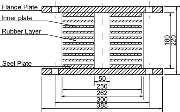
Figure 2.2.1 Configuration of thick rubber bearing
