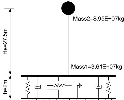
Fig.2.1.1 Simplified NPP model
