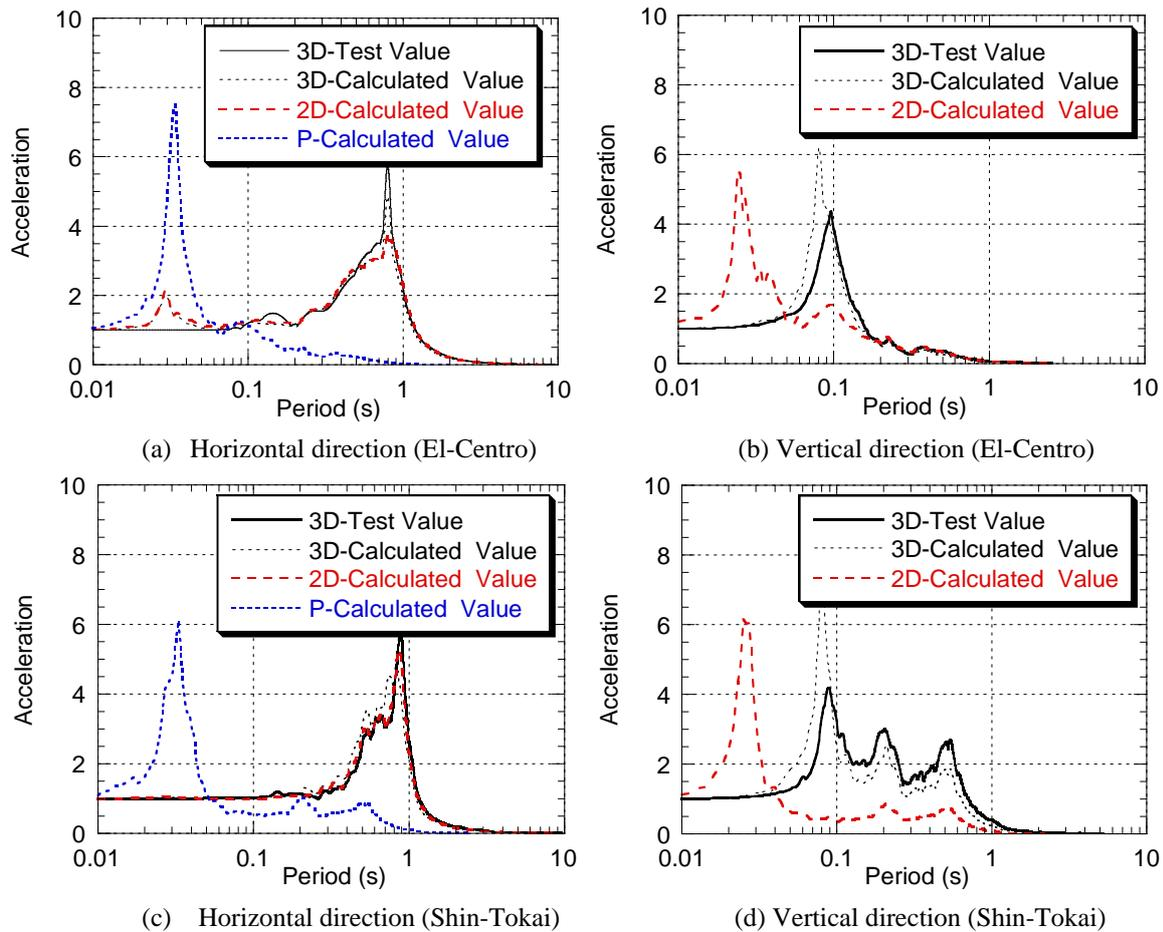
**Figure 3.4.2** Floor response spectrum contrast among three different models
