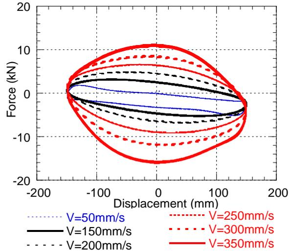
Figure 2.2.4 Energy dissipation capability
