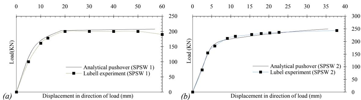
**Figure 6.** Pushover curves for strip model (see section 5.1) and Lubell (1997) test. (a) SPSW1; (b) SPSW2
