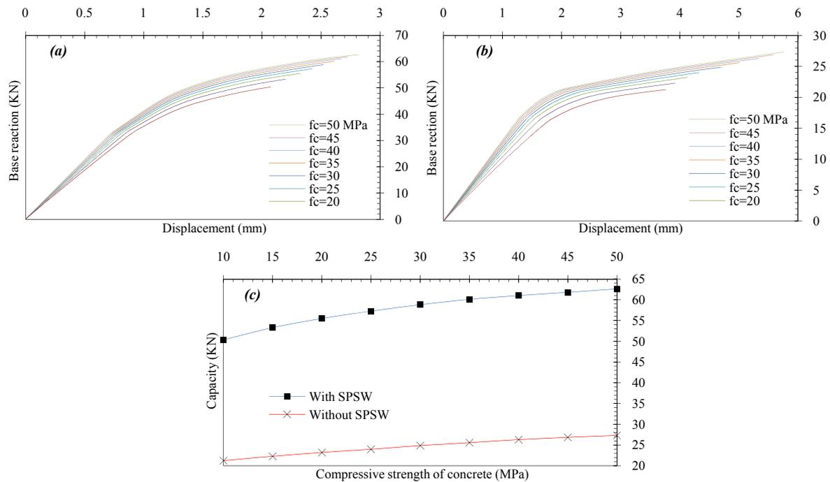
**Figure 10.** Analytical results (a) Pushover curves of different compressive strength (retrofitted concrete frame); (b) Pushover curves of different compressive strength (not retrofitted concrete frame); (c) Influence of compressive strength changes on capacity for two cases.
