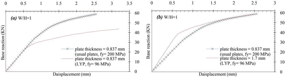
**Figure 8.** Analytical results (a) Pushover results for the frames retrofitted by LYP and normal steel plate with same thicknesses; (b) Pushover results for the frames retrofitted by LYP and normal steel plate (LYP thickness is twice of the normal plate thickness)
