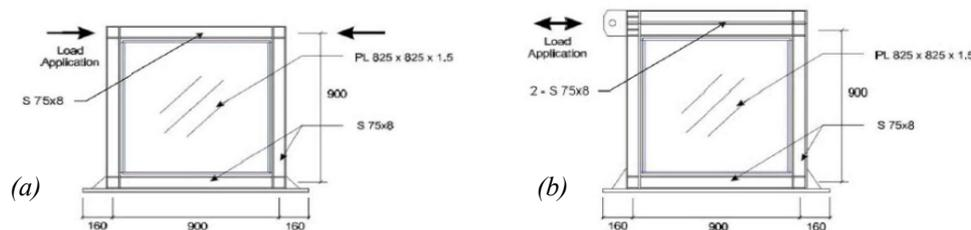
**Figure 2.** One-story test specimens (Lubell 1997): (a) SPSW1; and (b) SPSW2
