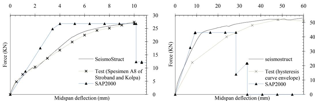
Figure 13. (a) Capacity curves for Specimen A8; (b) Capacity curves for Ghaffarzadeh *et al.* (2006) test.
