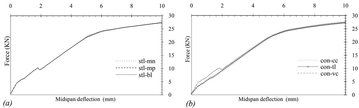
**Figure 3.** Comparison of SeismoStruct material models. (a) Steel; (b) Concrete.
