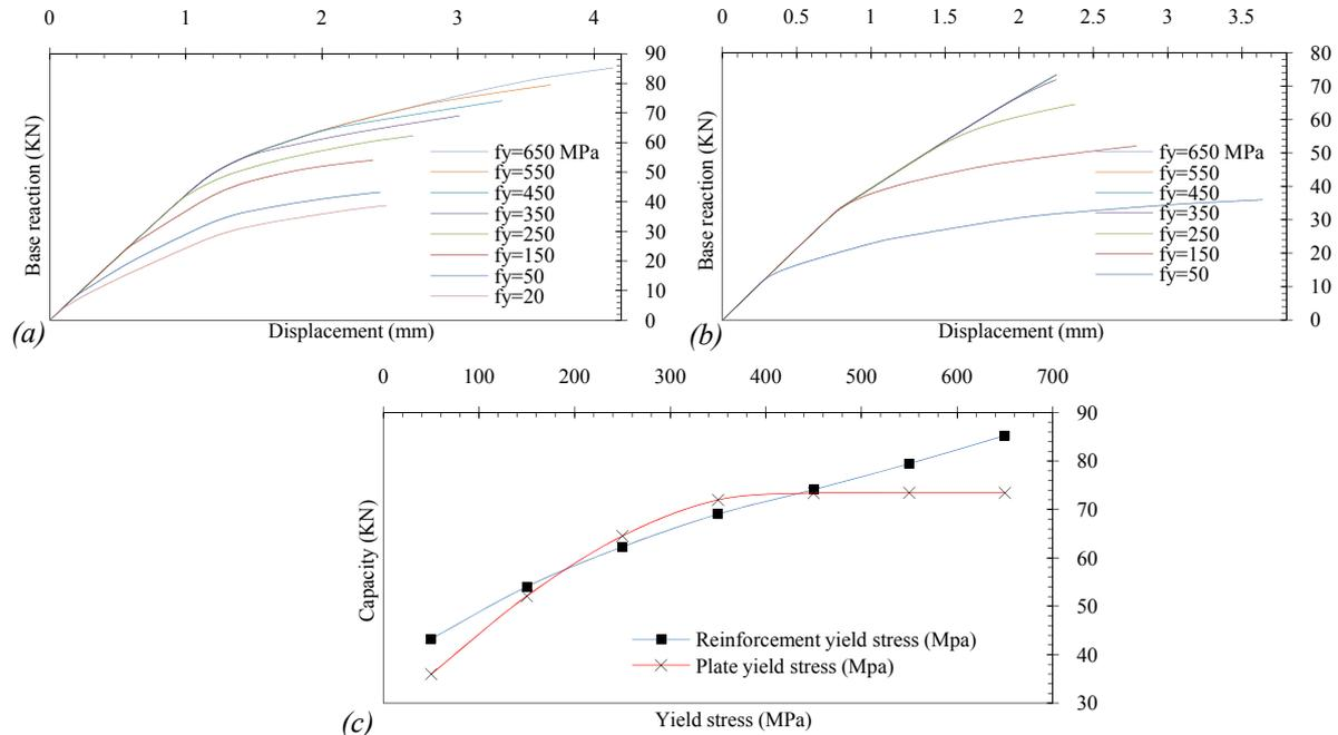
**Figure 7.** Comparison of change in capacity versus yield stress changing.
