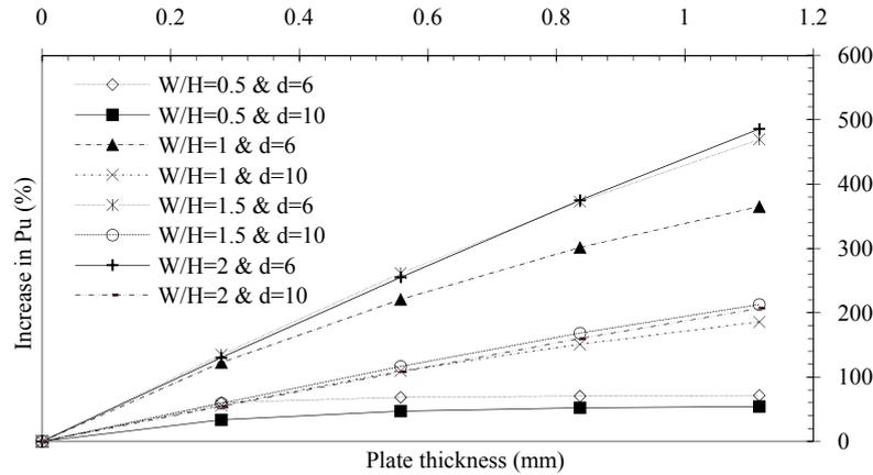
Figure 12. Increase of  $p_u$  versus plate thickness for RC frames strengthened by SPSW.
