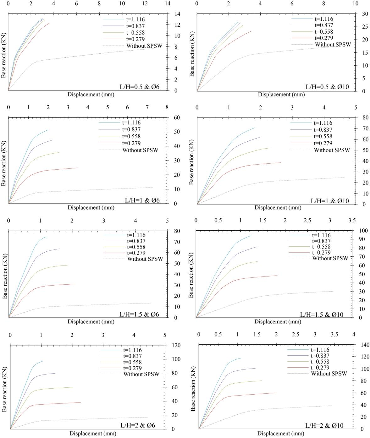
**Figure 11.** Effect of the parameters on behavior of the Retrofitted and not Retrofitted Frames
