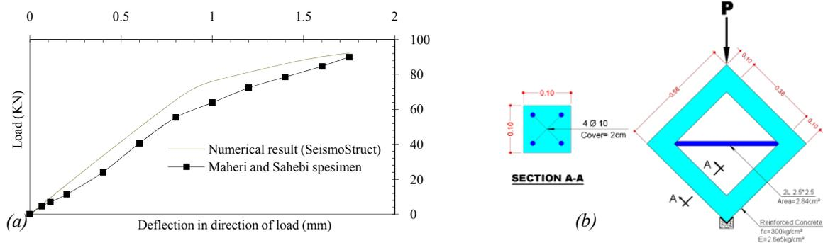
**Figure 5.** (a) Pushover curves for seismostruct model and Maheri *et al.* (1997) specimen; (b) Test set up and concrete frame geometry (Maheri *et al.* (1997))
