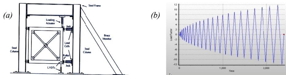
**Figure 1.** (a) Setup for cyclic testing of the model frames; (b) Detail of applied load (Ghaffarzadeh *et al.* 2006)
