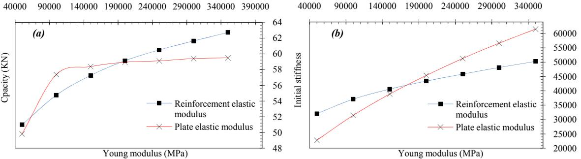
**Figure 9.** (a) Effect of plate and reinforcement module of elasticity on capacity; (b) Effect of plate and reinforcement module of elasticity on initial stiffness
