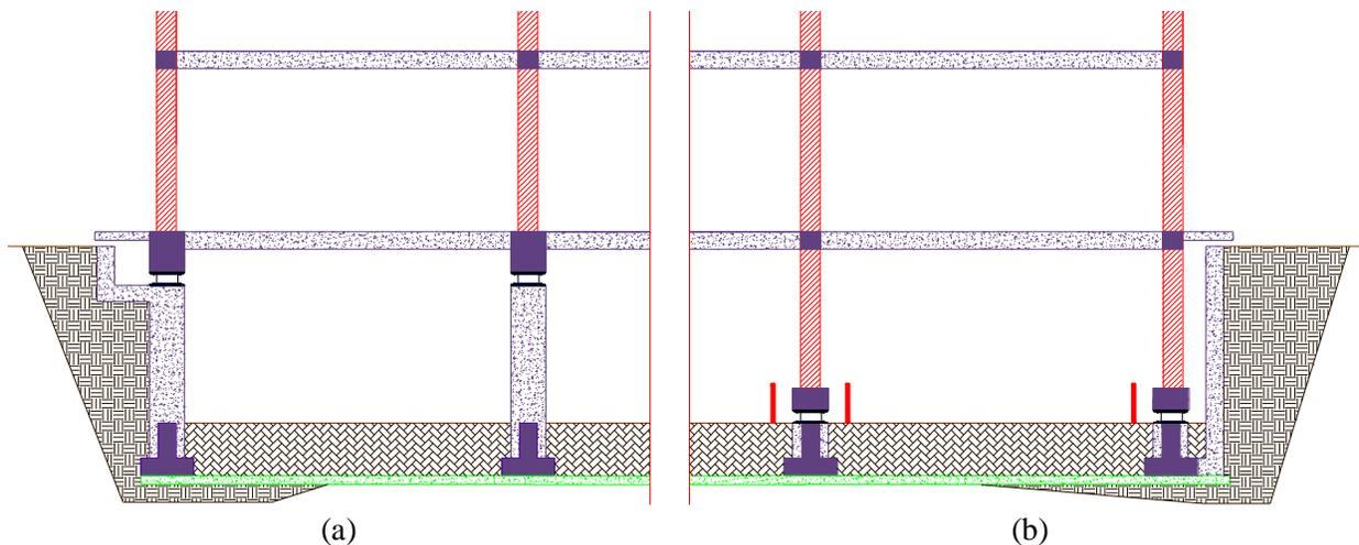
**Figure 3.2.** Isolation system (a) at the top and (b) at the base of the underground level
