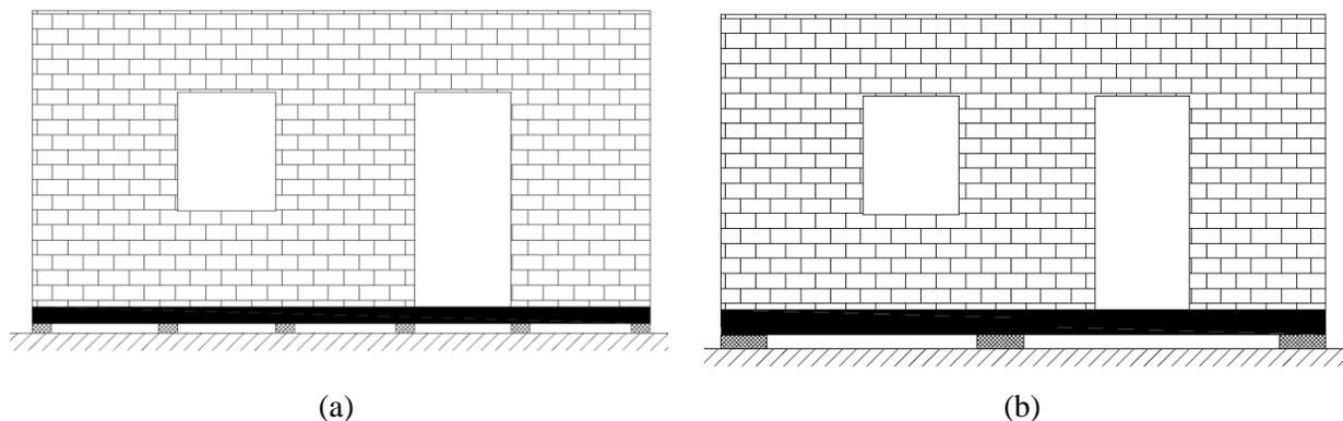
**Figure 3.1.** (a) Each masonry wall has at least two bearing, (b) isolator devices are at the wall crossings
