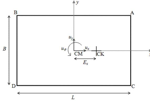
**Figure 2.1.** Plan view of the in-plane eccentric system with the indication of the degrees of freedom
