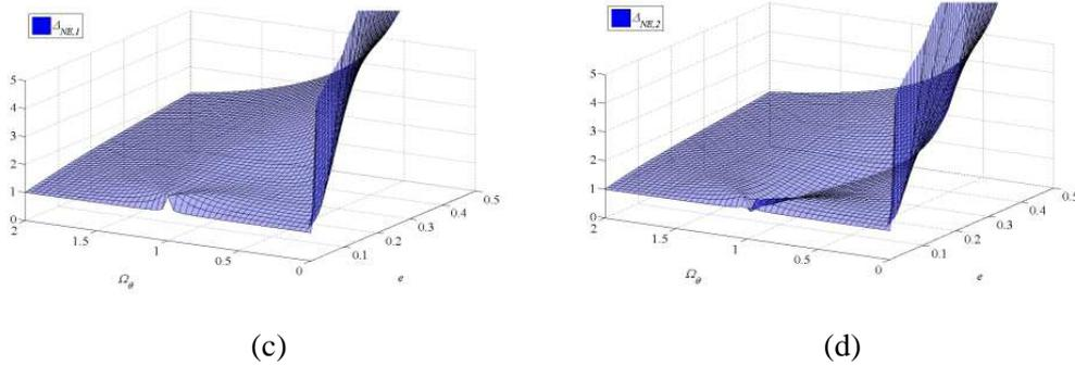
**Figure 6.1.** Corner displacement magnification with respect to: (a) center mass displacement based on HP1; (b) center mass displacement based on HP2; (c) center mass displacement of the equivalent N-E system based on HP1 (d) center mass displacement of the equivalent N-E system based on HP2
