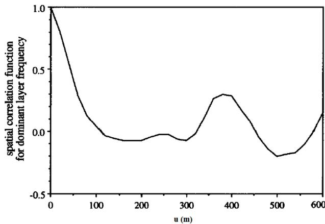
**Figure. 2.2.** Spatial autocorrelation function for the soil natural frequency estimated by Zerva & Harada (1997).
