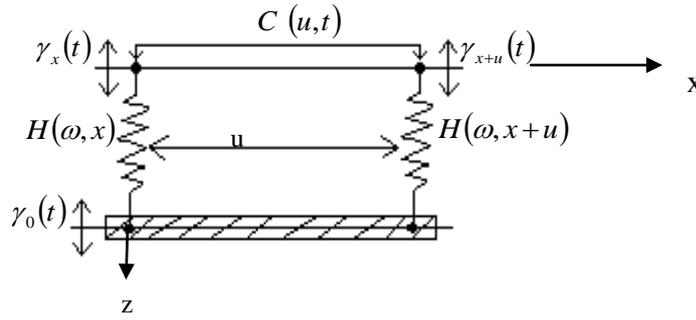
**Figure. 2.1.** Winkler model; case of a layer with stochastic properties.  $C(u,t)$  : inter correlation function,  $\gamma_0(t)$ : white process,  $\gamma_x(t)$  and  $\gamma_{x+u}(t)$ : filtered white process,  $H(\omega, x)$  and  $H(\omega, x+u)$  : transfer functions.
