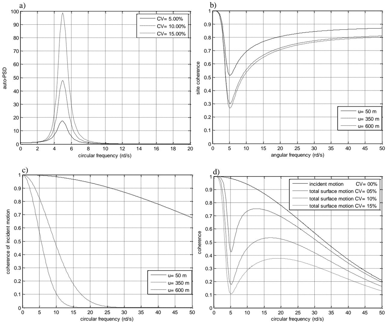
**Figure. 2.3.** a) Auto-PSD functions of site effect at various values of CV. b) Coherence of site effects at various separation distances. c) Loss of coherence of incident motion at various separation distances. d) Loss of total coherence at various values of CV.  $u=100\text{m}$ .
