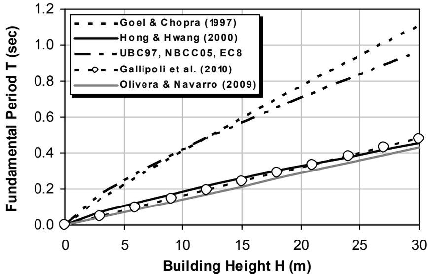
**Figure 3.** Comparison between Code, Goel & Chopra (1997) and the results of empirical studies based on ambient vibration measurements.
