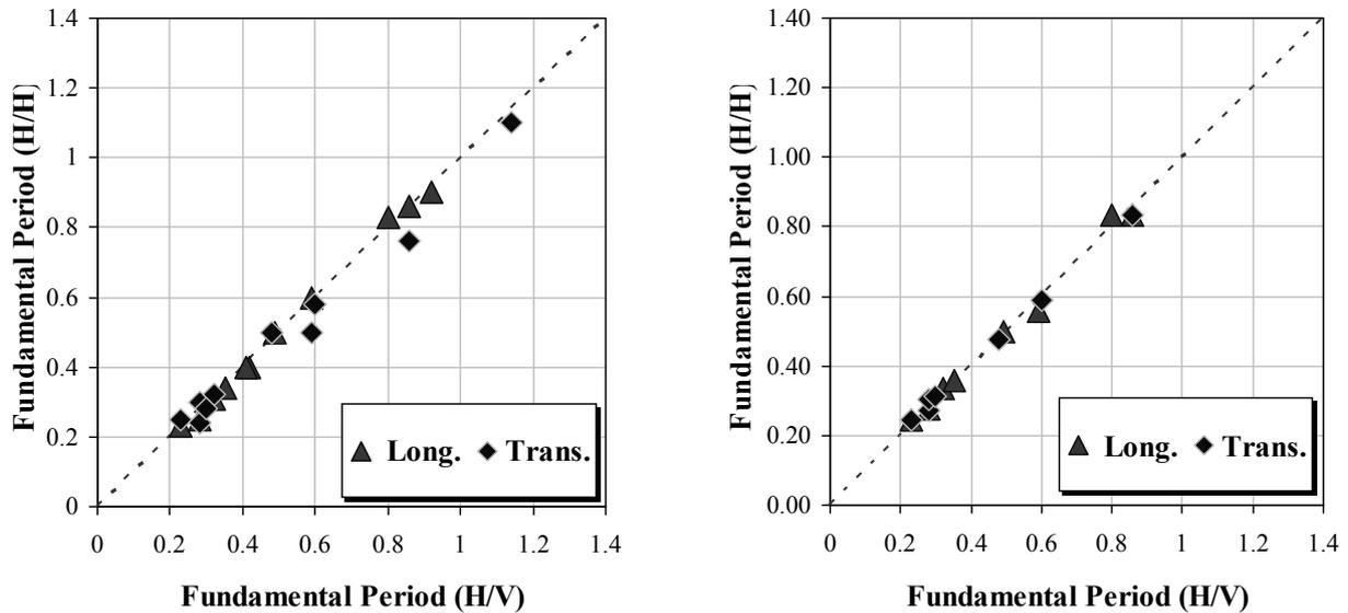
**Figure 6.** On the left: comparison between the fundamental periods estimated from HVSR and HHSR (measure on the basement) techniques for the two orthogonal directions (see text for details). On the right: comparison between the fundamental periods estimated from HVSR and HHSR (measure on free-field) techniques for the two orthogonal directions (see text for details).
