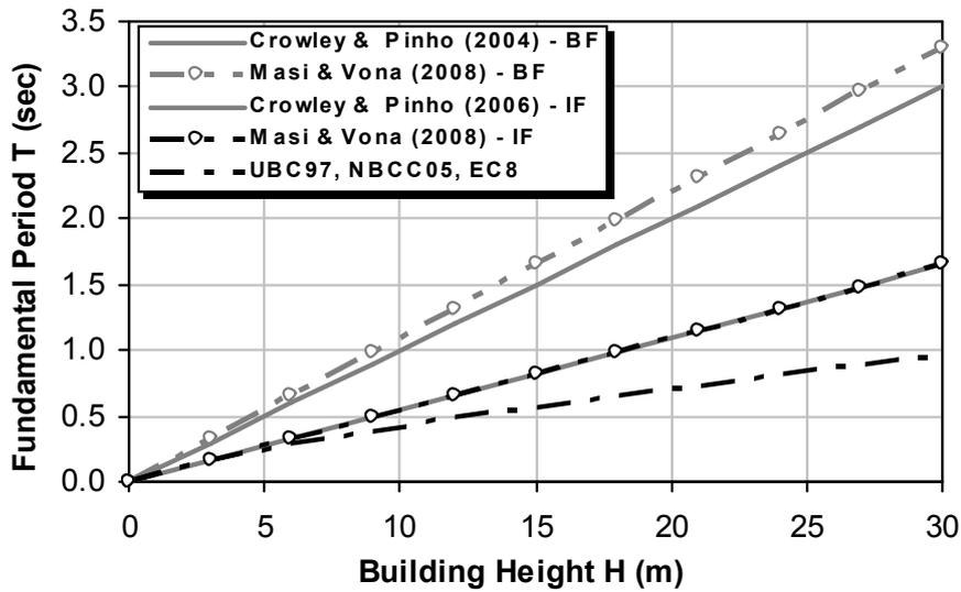
**Figure 1** Estimation of fundamental period of RC buildings having frames with (IF, Infilled Frame) and without (BF, Bare Frame) infills walls. Comparison with Code (UBC97, NBCC05, EC8) provisions.
