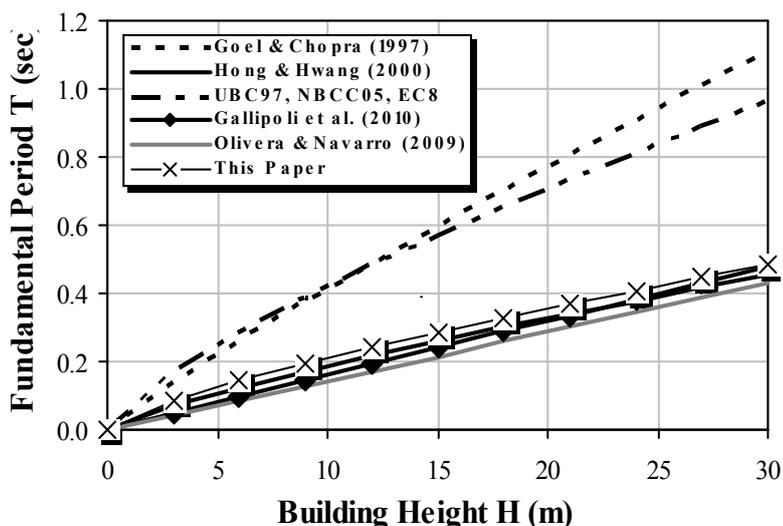
**Figure 9.** Comparison among period-height relationships. The empirical values based on ambient noise vibration are selected from Gallipoli *et al.* (2010), Oliveira & Navarro (2009) and BC Canada (this paper). The empirical values based on earthquake vibration are derived from Goel & Chopra (1997) and Hong & Hwang (2000). The theoretical relationships are the provision from EuroCode 8 (equal to UBC and NBCC2005).
