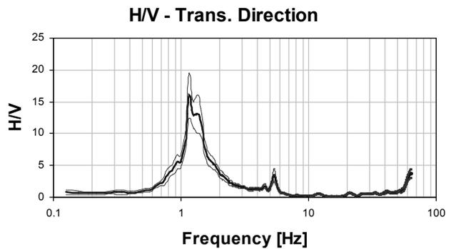
**Figure 5.** On the left: Student House in Vancouver. On the right: HVSR curves for the ambient vibration signals recorded on the longitudinal (Long) and transversal (Trans) direction of monitored building as a function of the vibration frequency. The mean value of H/V has been reported with  $\pm 1\sigma$  (standard deviation).
