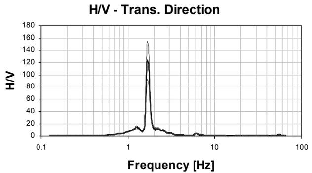
**Figure 4.** On the left: Marriott Hotel in Victoria. On the right: HVSR curves for the ambient vibration signals recorded on the longitudinal (Long) and transversal (Trans) direction of monitored building as a function of the vibration frequency. The mean value of H/V has been reported with  $\pm 1\sigma$  (standard deviation).
