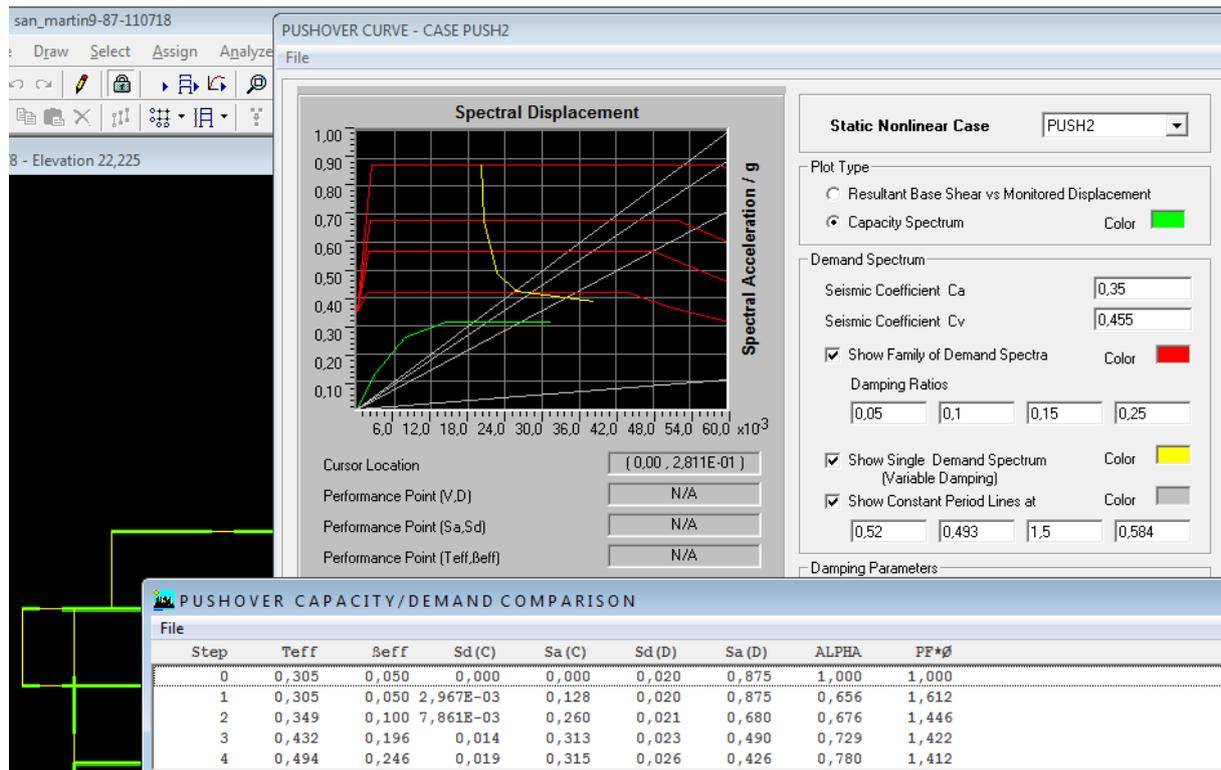
Figure 9. Capacity-Demand spectrum for the rare earthquake, x direction.
