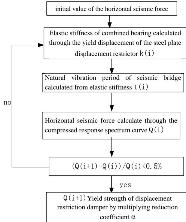
**Figure 2.** Design procedure of displacement restrictor
