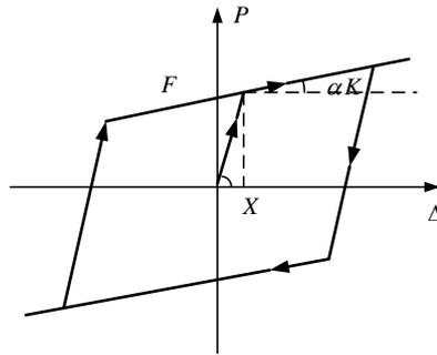
**Figure 1.** Calculation model of X shape steel plate constitution relationship
