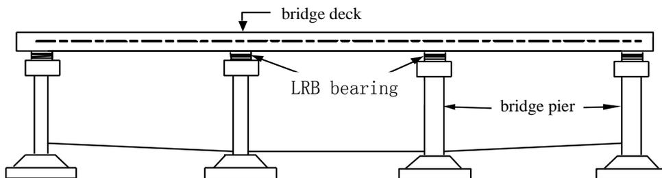
**Figure 3.** Sketch of seismic isolation bridge
