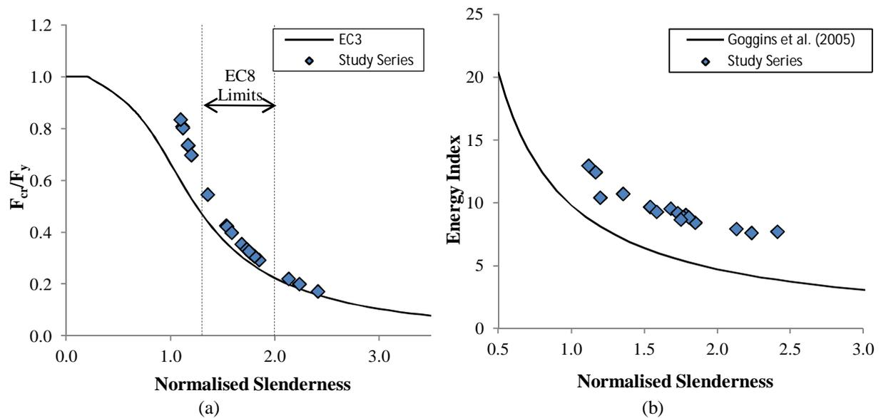
**Figure 4.4.** Normalised system slenderness versus (a) normalised critical load and (b) normalised hysteretic energy (energy index)
