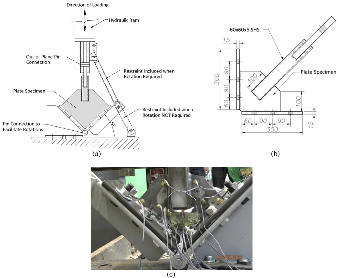
**Figure 2.1.**(a)-(c): (a) Test setup of specimen showing position of pin to allow plate rotations, (b) details of gusset plate specimen SP3a and (c) specimen SP3a after fracture.
