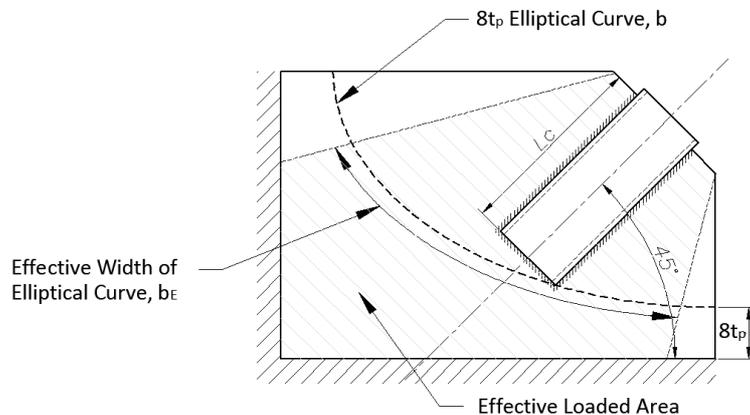
**Figure 4.2.** Gusset plate highlighting the effective loaded zone
