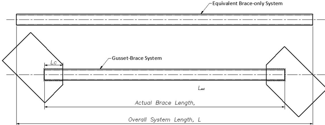
**Figure 4.3.** Comparison of gusset-brace system to equivalent brace-only system
