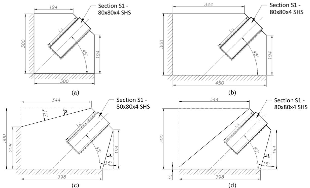
**Figure 4.1.** (a)-(d): Selected study specimens taken from full range of 12 (a) GP04, (b) GP05, (c) GP09, (d) GP11
