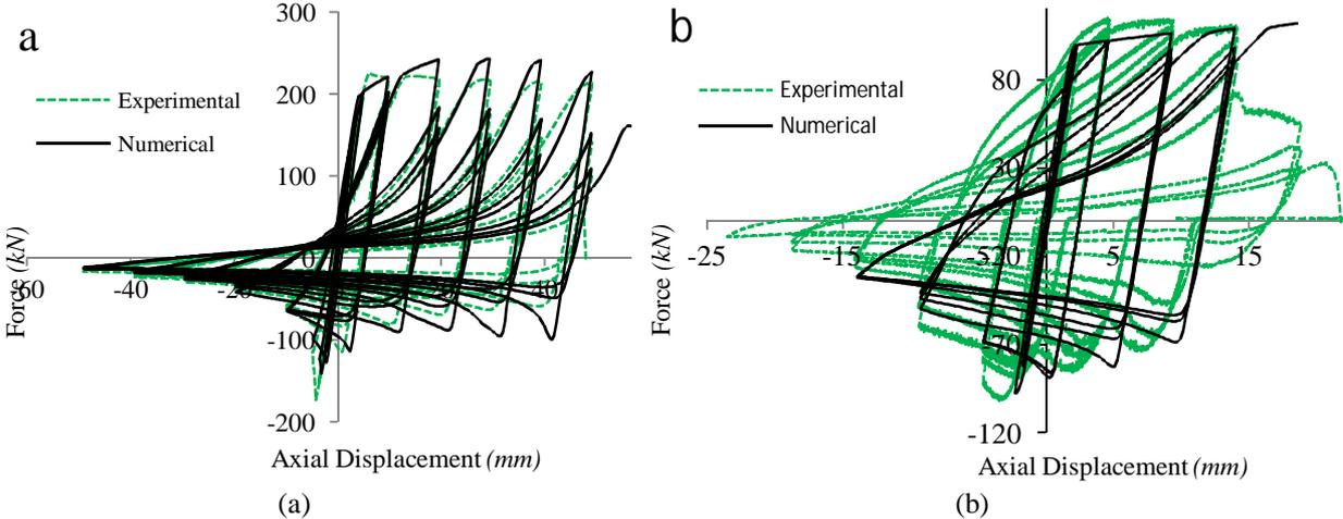
**Figure 3.1.** (a)-(b): Experimental hysteretic brace response of (a) 40x40x3x2050-CS-HR-Nip and (b) 40x40x2.5x1100-CS-CF-Goggins.
