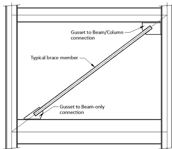
**Figure 1.1.** Typical CBF showing both a beam-column and a beam-only gusset connection.
