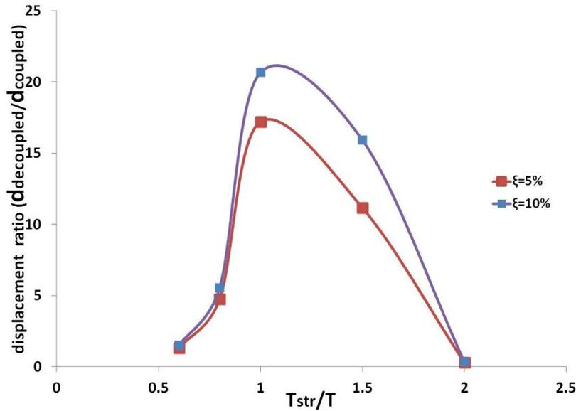
**Figure 4.** Ratio of decoupled displacements to coupled displacements of a sliding reinforced SDOF system for various values of the tuning ratio  $\beta=T_{str}/T$ . Damping ratio ( $\xi$ ) is equal to 5% and 10% and yield acceleration ratio ( $\tan\phi * g/a_{max}$ ) equal to 0.5.
