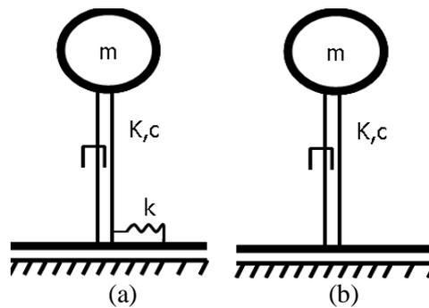
**Figure 2.** (a) Reinforced SDOF model, and (b) unreinforced SDOF model.
