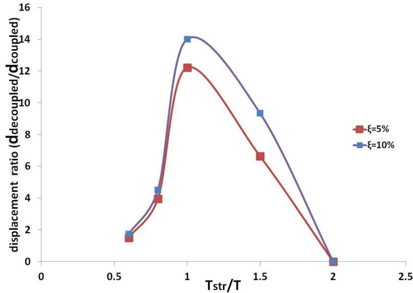
**Figure 6.** Ratio of decoupled displacements to coupled displacements of a sliding reinforced SDOF system for various values of the tuning ratio  $\beta=T_{str}/T$ . Damping ratio ( $\xi$ ) is equal to 5% and 10% and yield acceleration ratio ( $\tan\phi^*g/a_{max}$ ) equal to 1.0.
