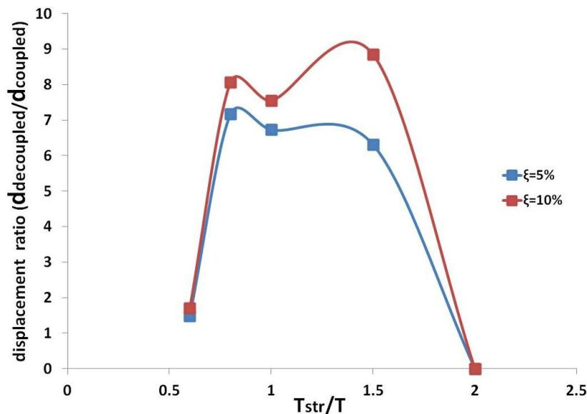
**Figure 5.** Ratio of decoupled displacements to coupled displacements of a sliding unreinforced SDOF system for various values of the tuning ratio  $\beta=T_{str}/T$ . Damping ratio ( $\xi$ ) is equal to 5% and 10% and yield acceleration ratio ( $\tan\phi * g/a_{max}$ ) equal to 1.0.
