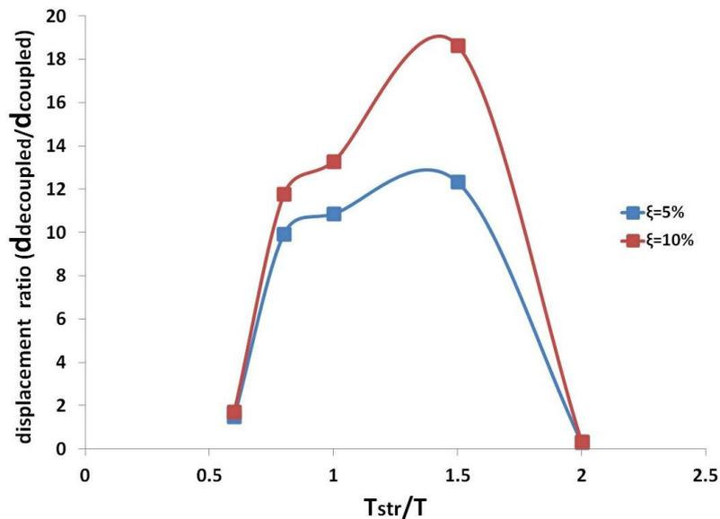
**Figure 3.** Ratio of decoupled displacements to coupled displacements of a sliding unreinforced SDOF system for various values of the tuning ratio  $\beta=T_{\text{str}}/T$ . Damping ratio ( $\xi$ ) is equal to 5% and 10% and yield acceleration ratio ( $\tan\phi^*g/a_{\max}$ ) equal to 0.5.
