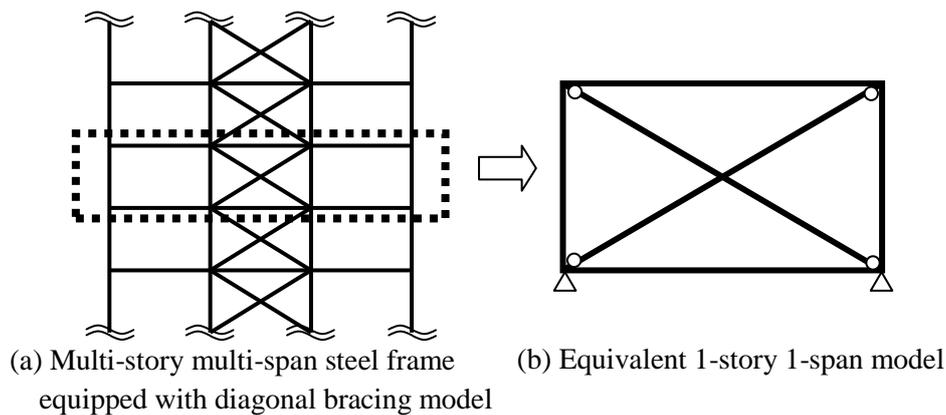
**Figure 3.1.** Analytical model of steel frame equipped diagonal bracing
