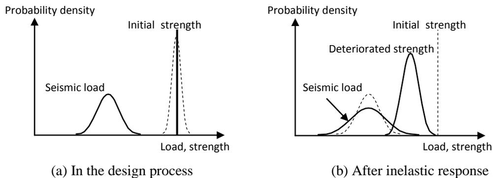
Figure 2.1. Performance evaluation curves in the design process and it after inelastic response behavior
