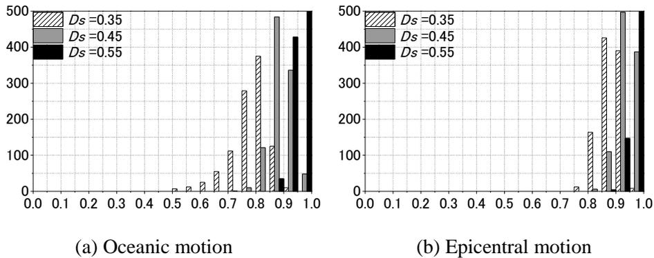
**Figure 4.2.** Statistical distribution of Residual ultimate strength ratio ( $R_{us}$ )
