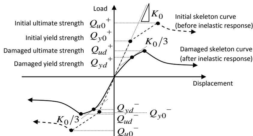
Figure 2.2. Skeleton curve of braced structure before and after inelastic response behavior
