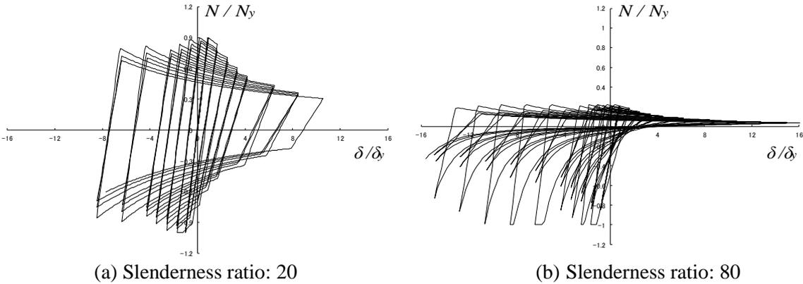
Figure 3.2. Model of restoring force characteristic of brace member
