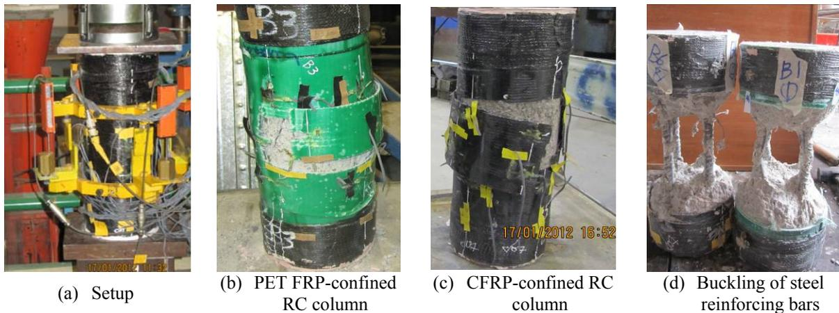
**Figure 4.** Test setup and failure mode
