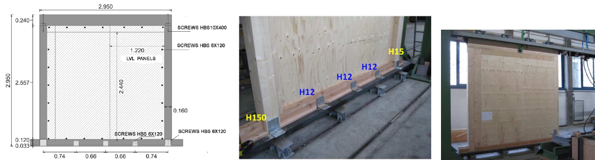
Figure 7. Geometry of the prototype - connection to the ground (steel angles type H150 and H120) and Dolomiti Plus prototype wall on the test bench
