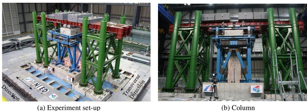
**Photo 1.** Experiment set-up using E-Defense shake table
