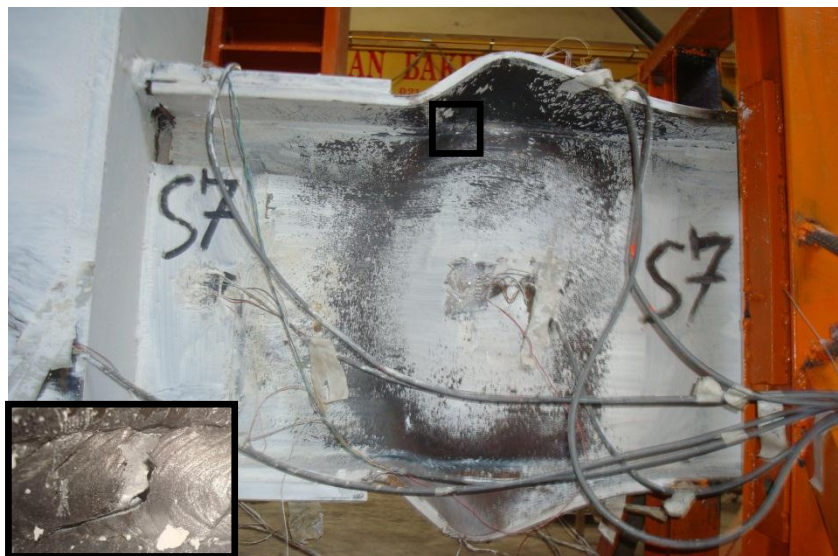
Figure 6. Fracture at the groove weld joining the beam web to the beam flange in the BD53
