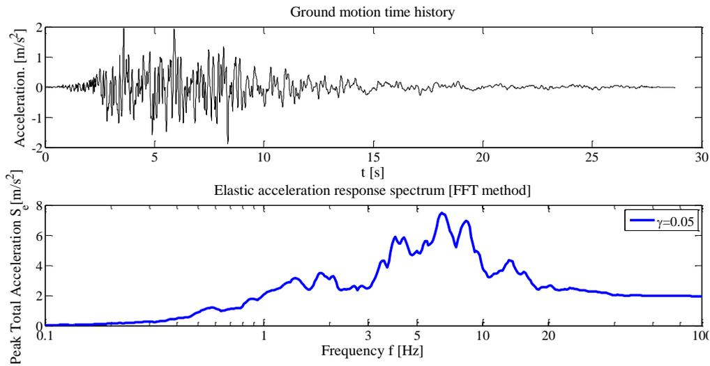
**Figure 3.2.** Ground motion time history (horizontal component) and its elastic acceleration response spectrum – Westmorland earthquake,  $\text{PGA}=1.95 \text{ [m/s}^2\text{]}$ .
