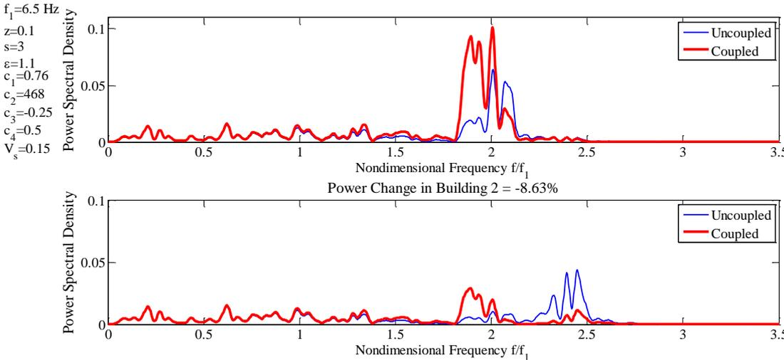
**Figure 4.2.** Response power spectra for total sway displacements for buildings 1 and 2 due to Westmorland earthquake.
