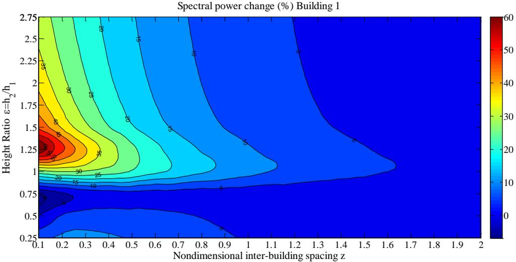
**Figure 4.6.** Change in power (caused by coupling) vs. height ratio  $\epsilon$  and inter-building spacing  $z$ ,  $s=3.25$  - Westmorland.
