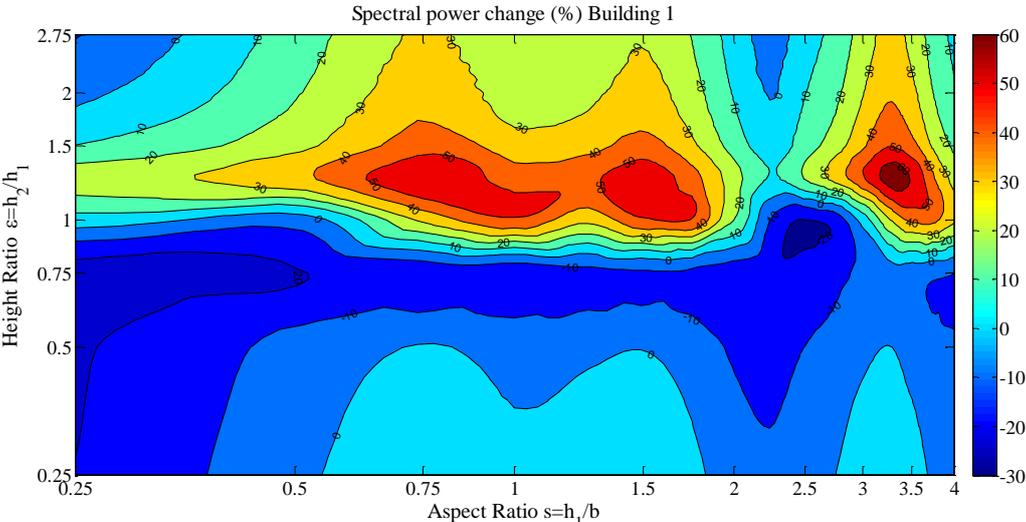
**Figure 4.4.** Change in power (caused by coupling) vs. aspect and height ratio caused by Westmorland.
