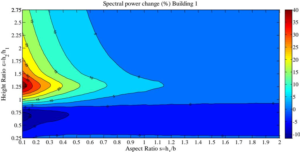
**Figure 4.5.** Change in power (caused by coupling) vs. height ratio  $\epsilon$  and inter-building spacing  $z$ ,  $s=3.25$  - Kanai-Tajimi
