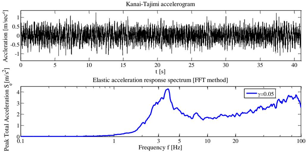
**Figure 3.1.** Kanai Tajimi artificial accelerogram and elastic acceleration response spectrum (5% damping).
