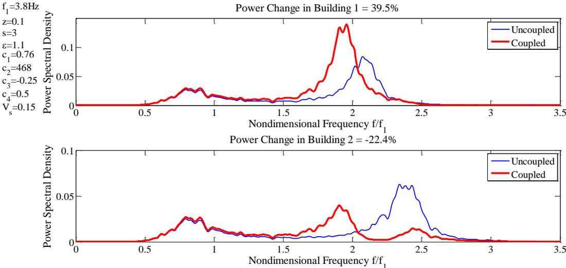
**Figure 4.1.** Response power spectra for total sway displacements for buildings 1 and 2, due to Kanai-Tajimi excitation.
