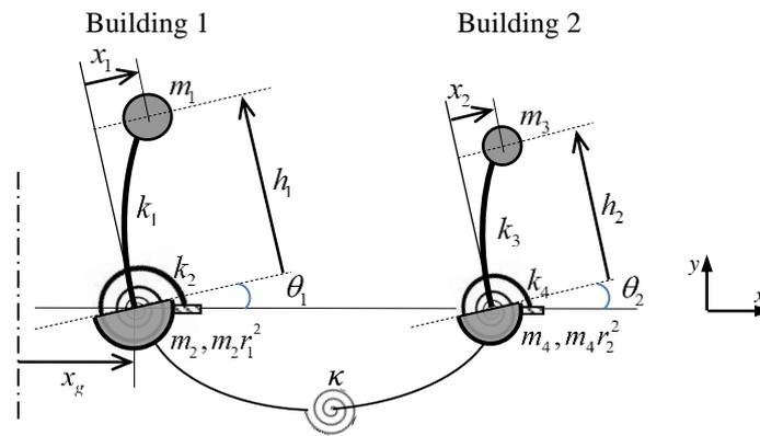
**Figure 2.1.** Two buildings discrete model
