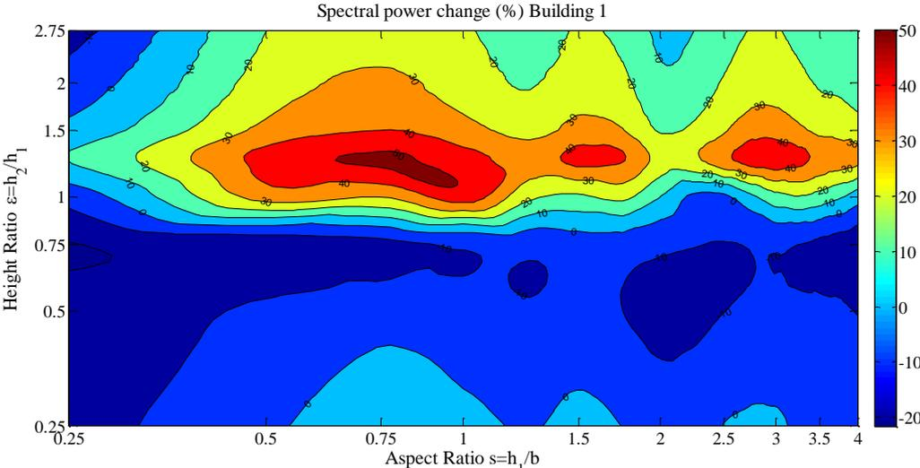
**Figure 4.3.** Change in power (caused by coupling) vs. aspect and height ratio caused by Kanai-Tajimi.
