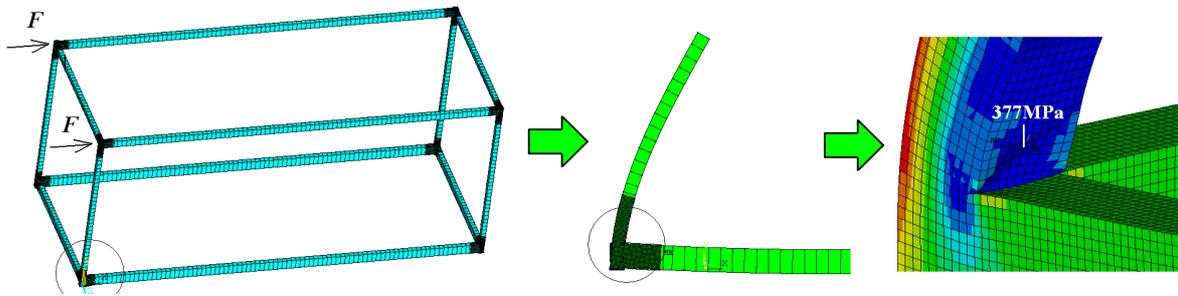
**Figure 6.** Typical MSCF failure in a column of modular frame
