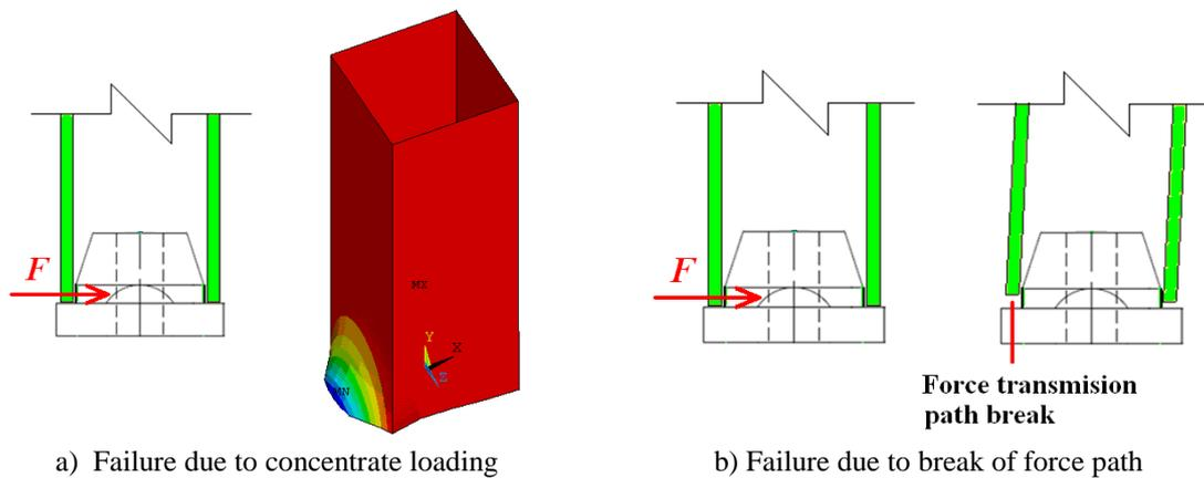
**Figure 7.** Typical LCF at the connection region between modular units
