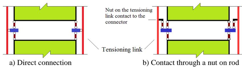
**Figure 4.** Connection between tie rods and connectors
