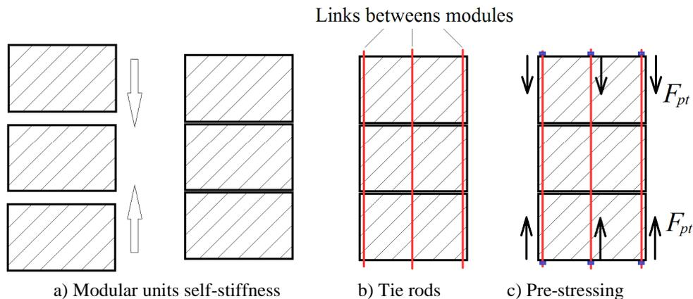
**Figure 2.** Schematic of a typical PTMS
