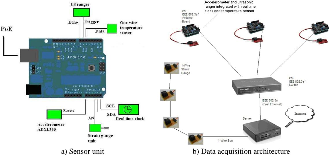
**Figure 9.** Architecture of sensor unit based on Arduino Uno and data acquisition system
