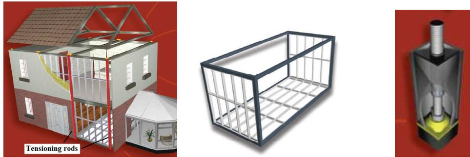
**Figure 1.** Building structure made from modular units and tie rods (courtesy Powerwall, 2008)
