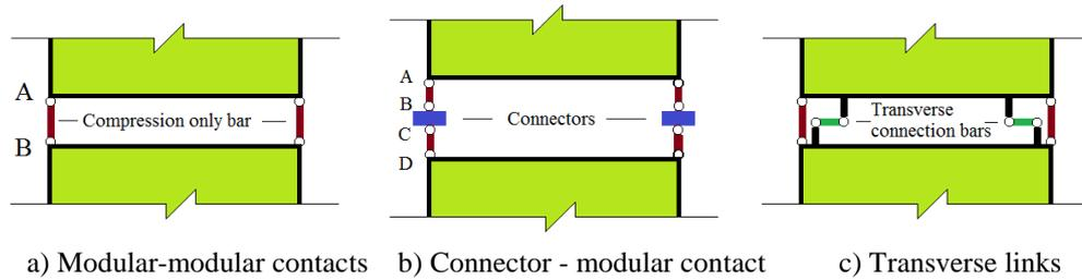
**Figure 3.** Connection between modules and connector
