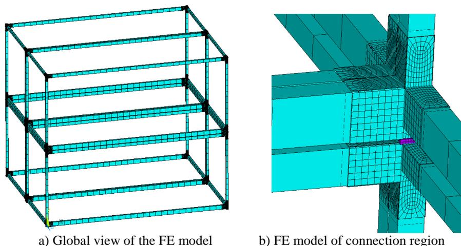
**Figure 5.** FE model of a typical modular frame with 4 modular units (2-bay, 2-storey)
