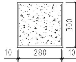
**Figure 2.3.** Cross section of the CFST specimen
