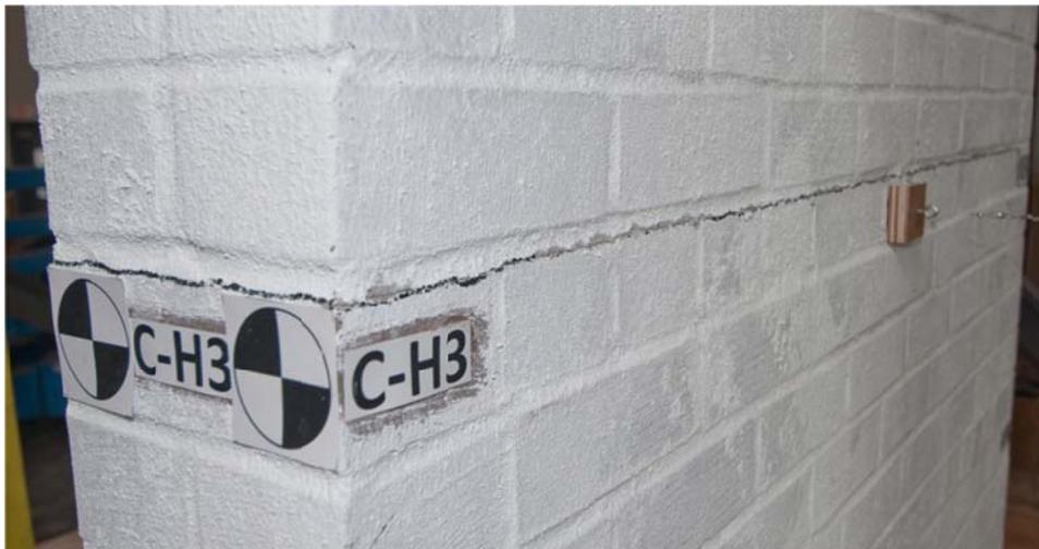
**Figure 7.** Crack in Wall C
