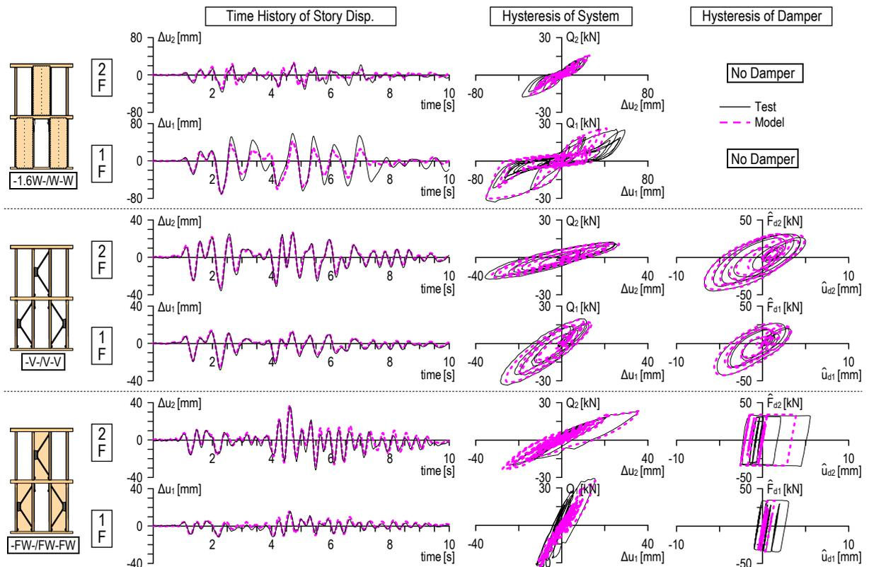
**Figure 12** Comparison of Test and Analysis of Global Behavior (2-Story Frame, JMAKobe0.6g)
