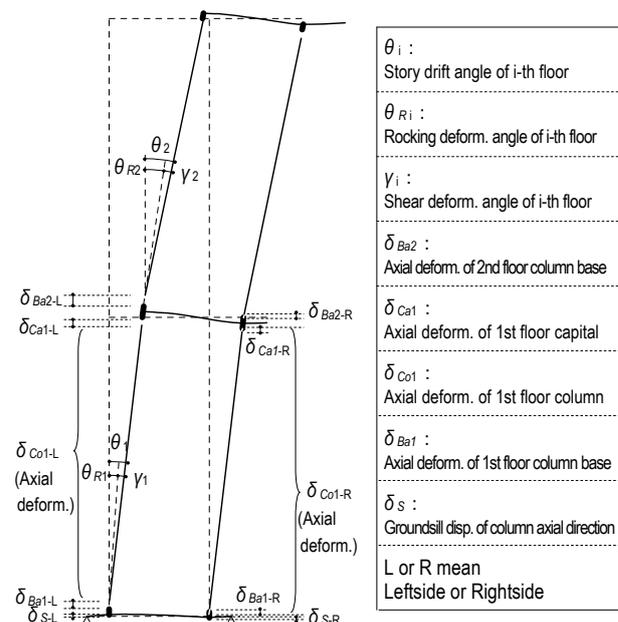
Figure 16 Deformed State and Definition of Symbol
