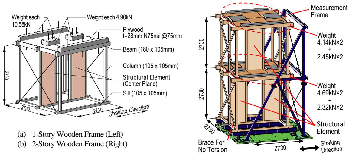
**Figure 10** Shake Table Test of Wood Frame with Damper
