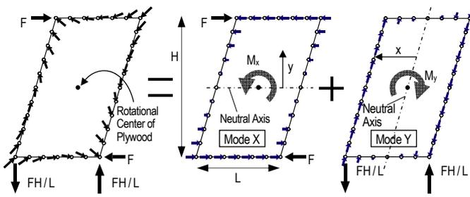
Figure 4 Force Acting on Frame (Elastic)
