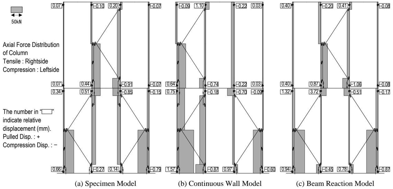
**Figure 15** Axial Force Distribution of Column and Relative Displacement of Joint at Peak Strength of 1st Floor
