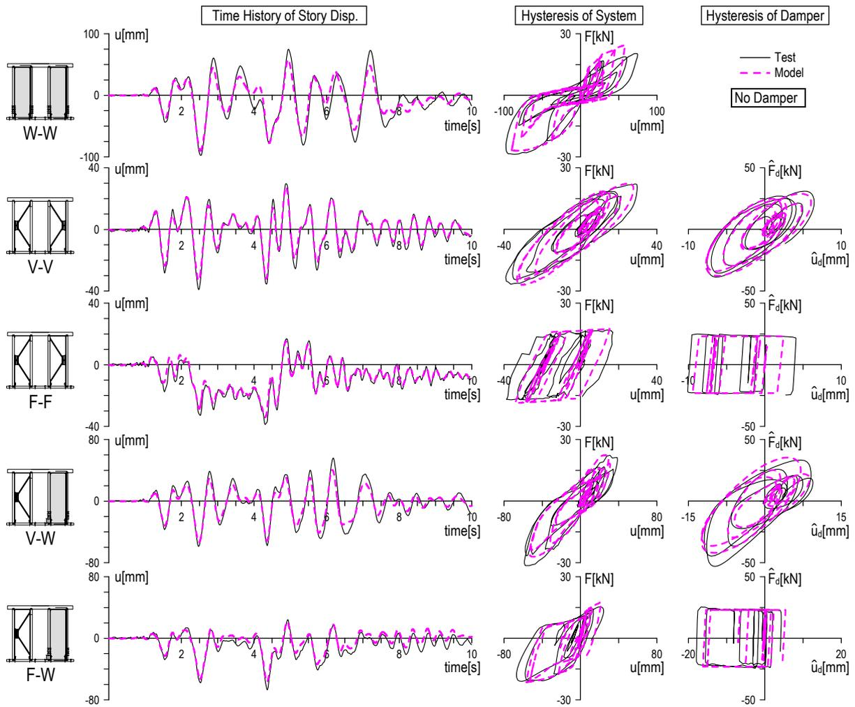
**Figure 11** Comparison of Test and Analysis of Global Behavior (1-Story Frame, JMAKobe0.6g)
