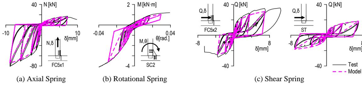
**Figure 7** Modelization Example of Joint between Column and Horizontal Member
