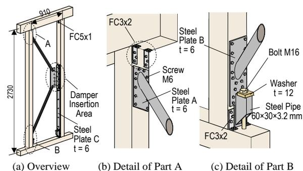
**Figure A1** Detail of Energy Dissipation Wall
