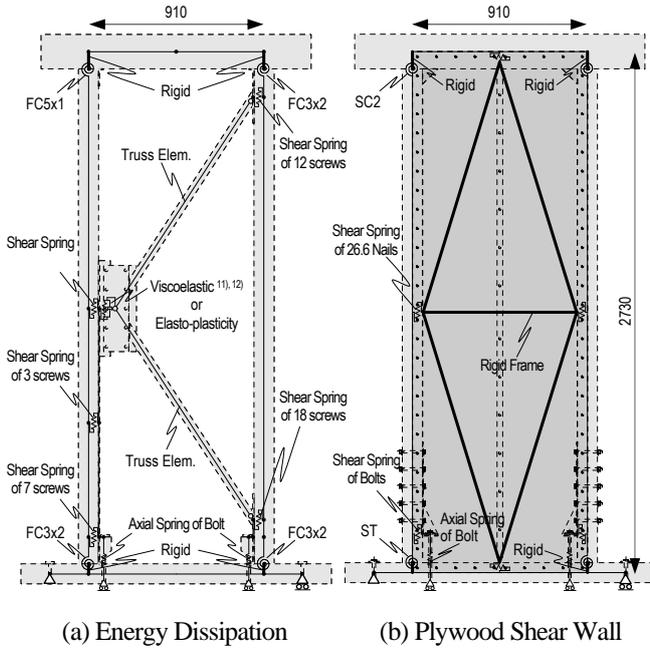
Figure 1 Detail of Frame Model
