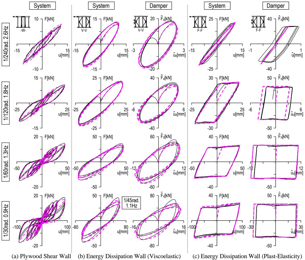
**Figure 9** Comparison of Test and Analysis of Cyclic Loading
