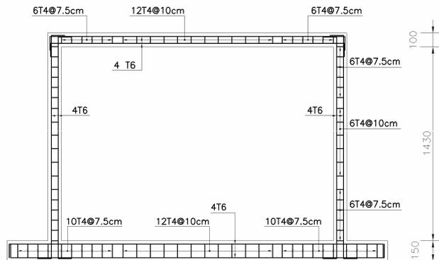
**Figure 3.** Reinforcement details of the wall specimens (dimensions in mm)
