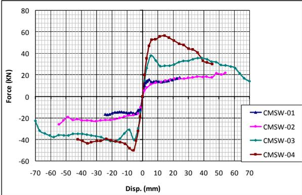
Figure 10. The envelopes of hysteresis curves of CMSW specimens
