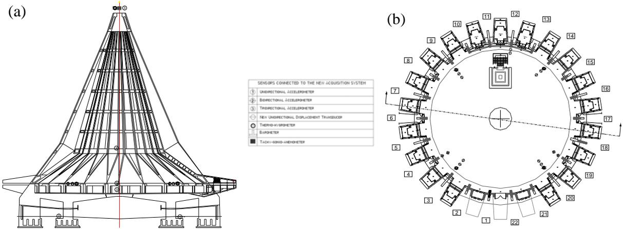
**Figure 1.2.** Vertical cross-section (a), plane at isolators' level (b) of the new monitoring system
