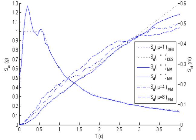
**Figure 3.2.** Design (DES) & mean matched (MM) acceleration and displacement constant  $\mu$  RS ( $\xi=5\%$ )
