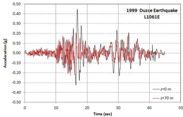
**Figure 10.** Time histories at surface ( $z=0$ ) and  $z=70$ m depth obtained from site response analysis at idealized soil profile in Van region with using Duzce earthquake ground motion record in E-W direction
