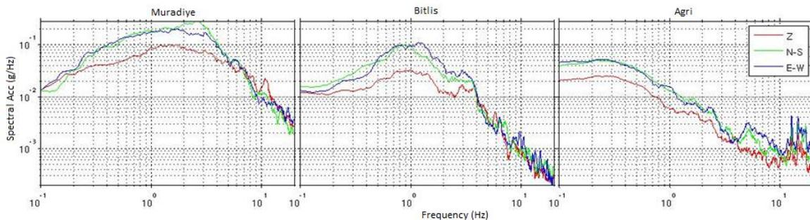
**Figure 14.** The acceleration amplitude spectra of the strong motion recordings at Muradiye, Bitlis and Agri stations
