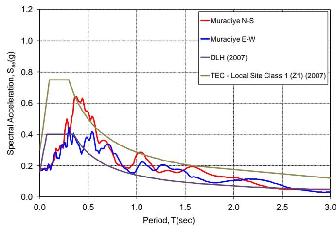
**Figure 15.** Response spectra of Van-Tabanlı earthquake of October 23, 2011
