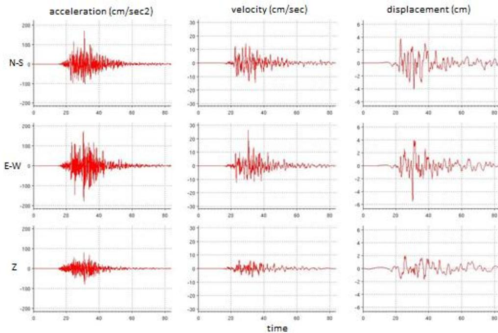
**Figure 13.** Acceleration, velocity and displacement time histories of the recordings of  $M_w=7.2$  earthquake at the Van- Muradiye station
