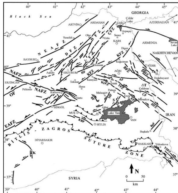
**Figure 2.** Main active faults in East Anatolia (NAFZ: North Anatolian Fault Zone, EAFZ: East Anatolian Fault Zone, EF: Ercis Fault, CF: Cildiran Fault (source of the M=7.5 earthquake in 1976)) (Bozkurt, 2001)
