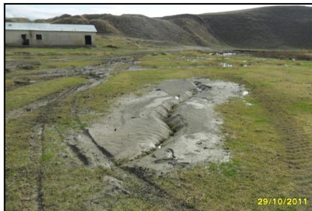
**Figure 7.** Sand boils due to liquefaction in Topaktas village, Van
