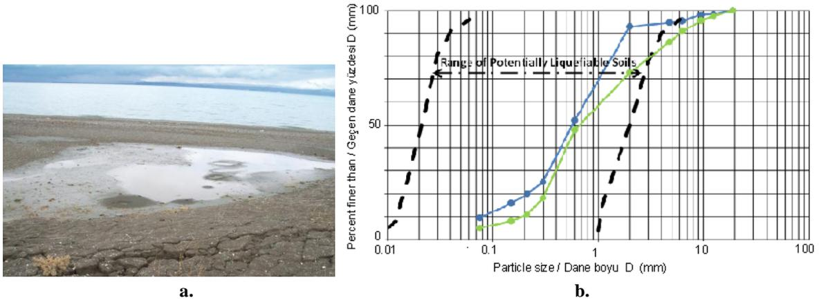
**Figure 8.** Lateral deformations: a. seismic soil liquefaction-induced sand boils and lateral spreading by Lake Van; b. sieve analysis
