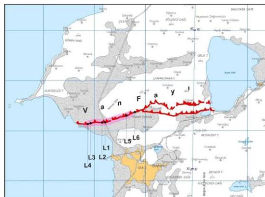
**Figure 3.** Surface rupture map of the October 23, 2011 Van earthquake (Emre *et al.* 2011) (pink line is the surface rupture)
