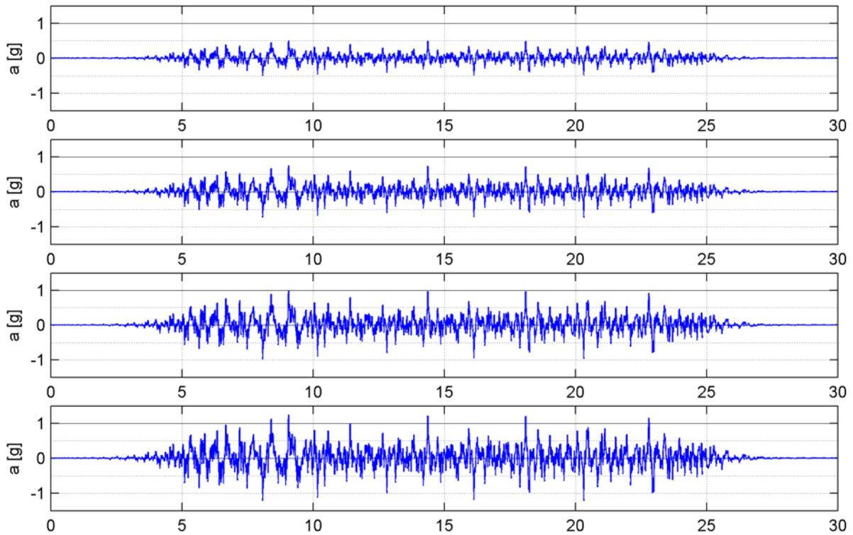
**Figure 2.4.** Input acceleration time histories for Y direction corresponding to SDS equal to 0.30g, 0.60g, 0.90g, 1.20g and 1.50g.
