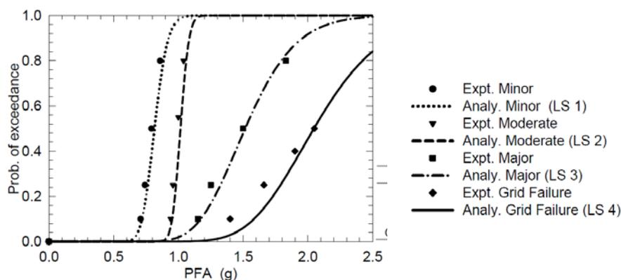
**Figure 3.2.** Ceiling fragility curve: ceiling with undersized tiles (Badillo-Almaraz et al. 2007)
