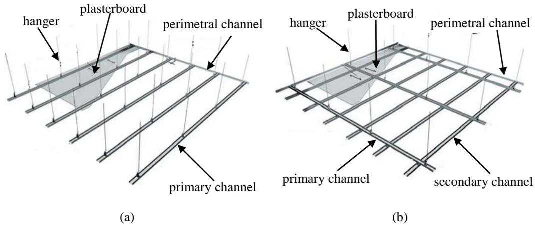
**Figure 2.1.** Suspended plasterboard continuous ceilings: (a) single frame ceiling (SFC); (b) double frame ceiling (DFC)
