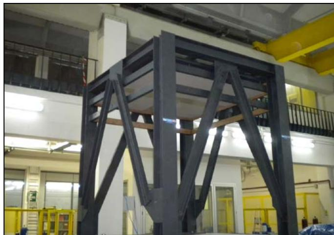
**Figure 2.2.** Test frame installed on the shake table
