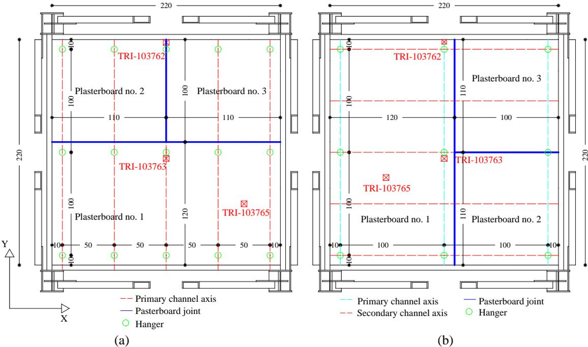
**Figure 2.3.** Triaxial accelerometers, plasterboard and hanger position in the case of single frame ceiling (a) and double frame ceiling (b) specimen
