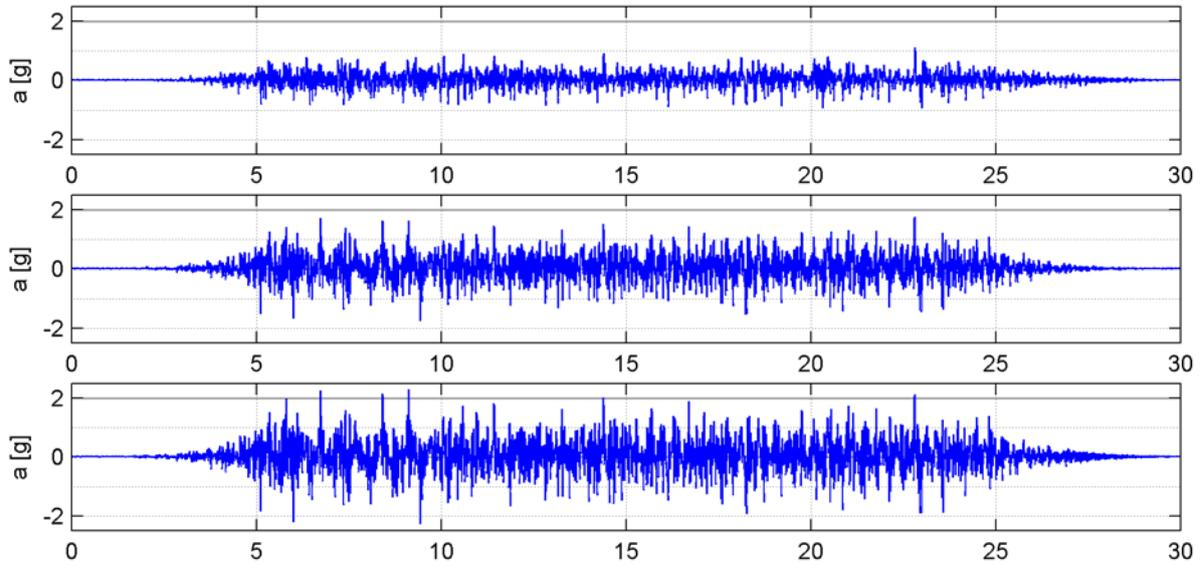
**Figure 3.1.** Acceleration time histories recorded on the ceiling (Accelerogram no. 103763) for single frame ceiling (SFC) for the intensity levels corresponding to SDS equal to 0.30g, 0.60g, 0.90g, 1.20g and 1.50g.
