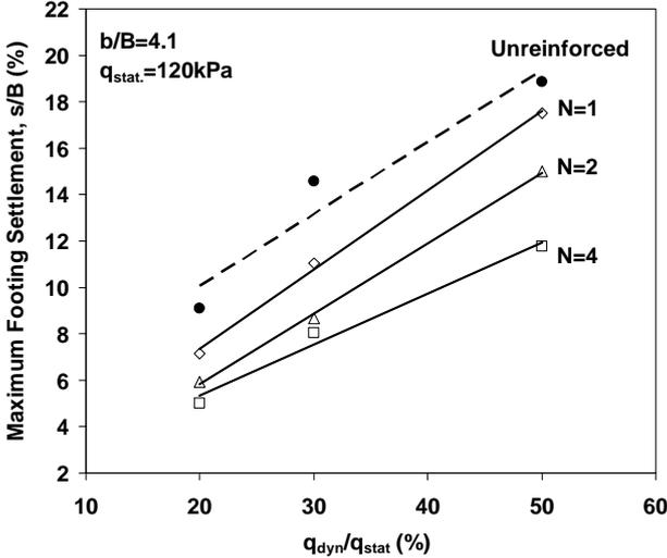
**Figure 3.** Variation of the maximum footing settlement ( $s/B$ ) with amplitude of repeated loads for unreinforced and reinforced bed.
