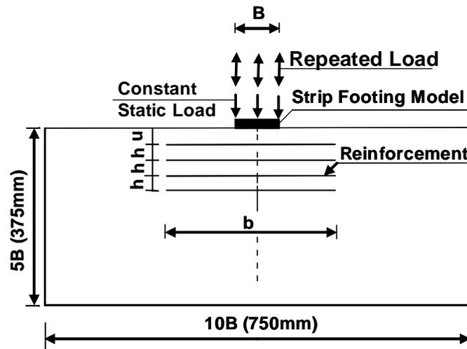
**Figure 1.** Geometry of the planar geotextile-reinforced foundation bed.
