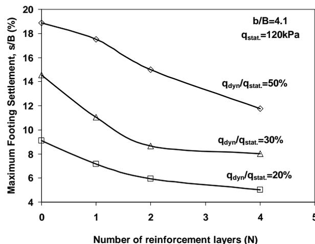
**Figure 5.** Variation of the maximum footing settlement ( $s/B$ ) with number of layers of reinforcements under repeated loading of amplitude  $q_{dyn}/q_{stat}=20\%$ ,  $30\%$  and  $50\%$ .
