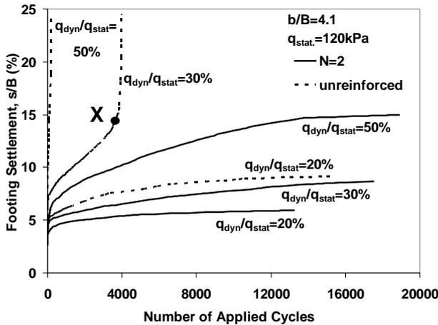
**Figure 2.** Variation of the footing settlement ( $s/B$ ) with number of applied load repetitions for the unreinforced and reinforced beds ( $N=2$ ).
