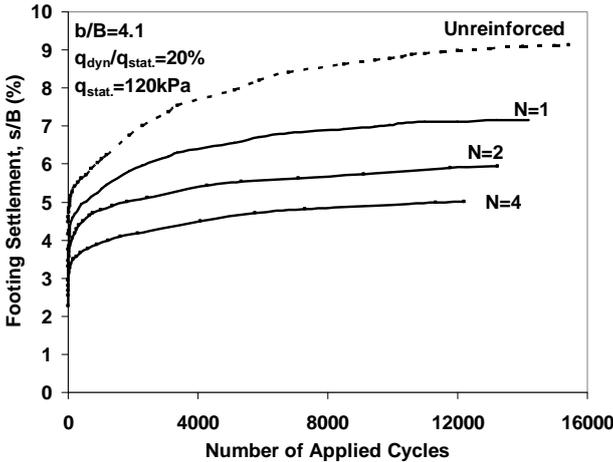
**Figure 4.** Variation of the footing settlement ( $s/B$ ) with number of applied load repetitions at  $q_{dyn}/q_{stat}=20\%$  for the unreinforced and reinforced beds.
