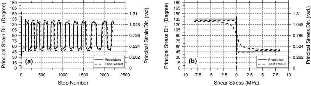
**Figure 6.** Principal strain and stress directions for Specimen SE10: (a) Principle strain direction history, (b) Principal stress direction in concrete vs. shear stress behavior
