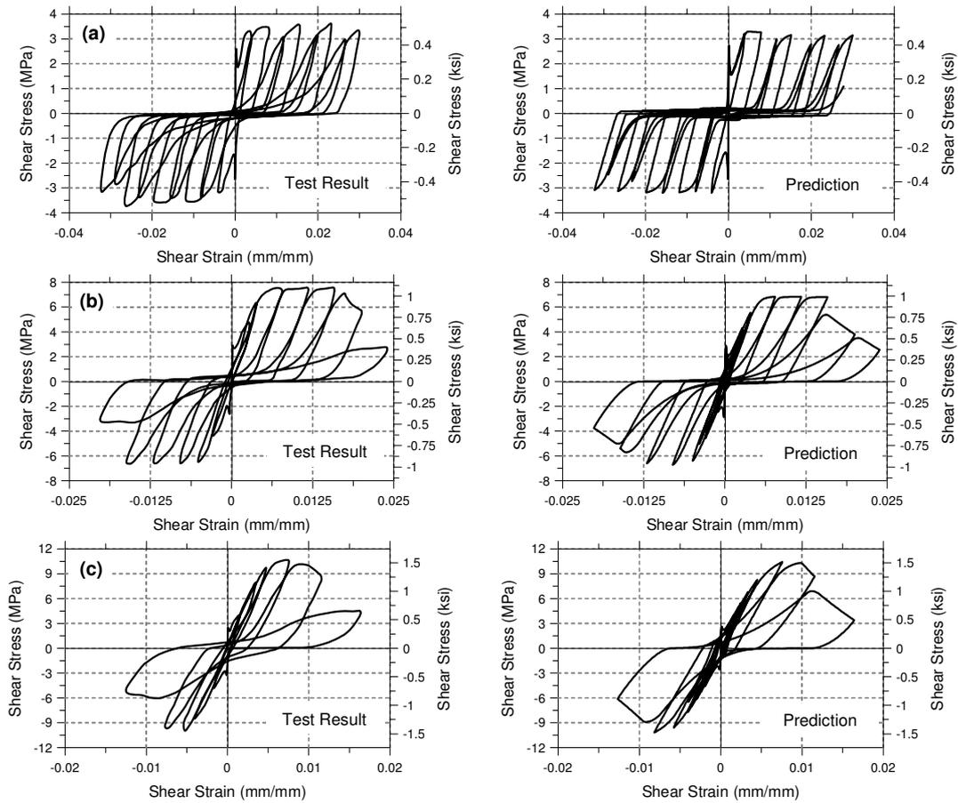
**Figure 7.** Comparison of measured and predicted shear stress vs. shear strain responses: (a) Specimen CA2, (b) Specimen CA3, (c) Specimen CA4
