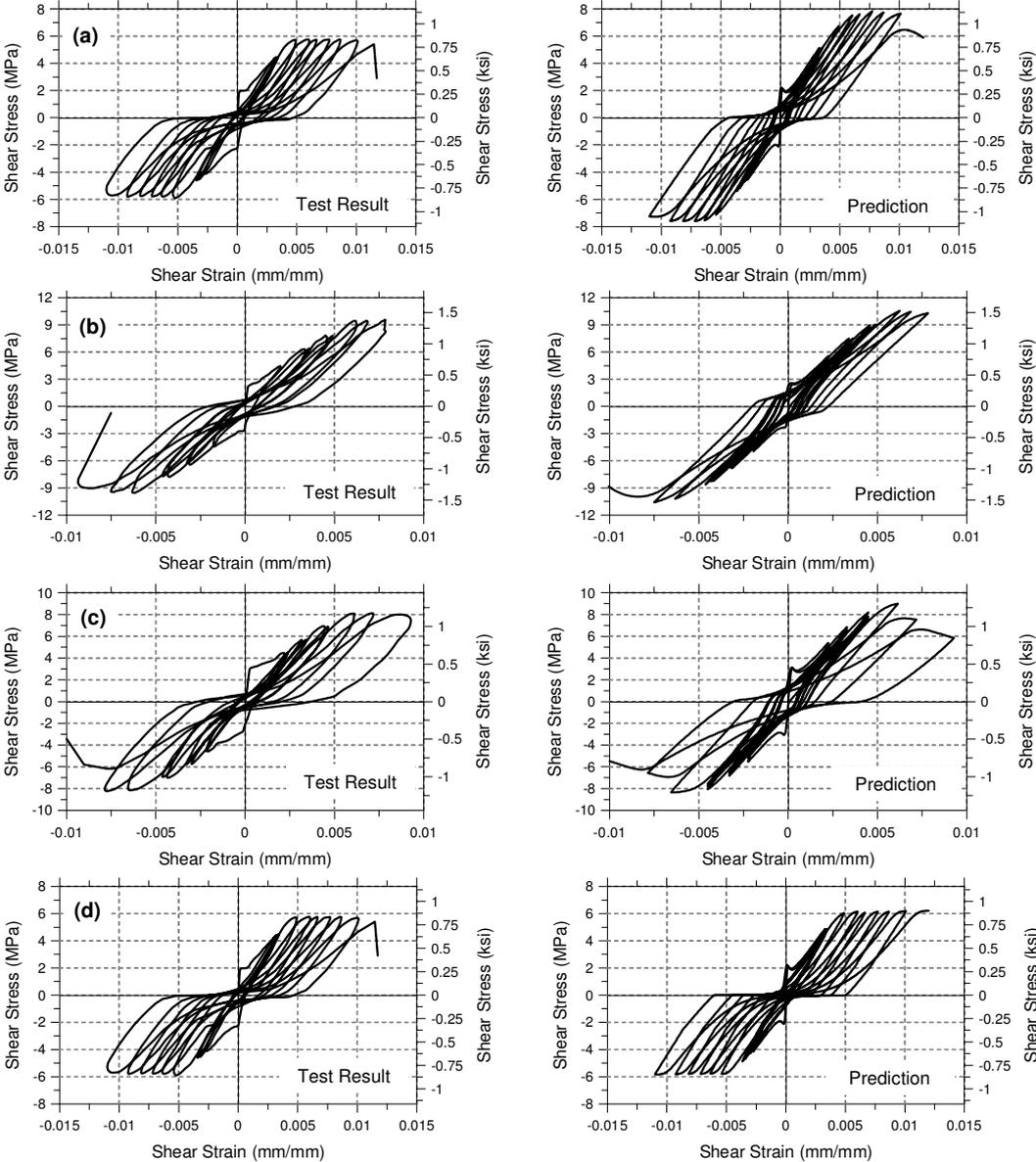
**Figure 4.** Comparison of measured and predicted shear stress vs. shear strain responses: (a) Specimen SE8, (b) Specimen SE9, (c) Specimen SE10, (d) Specimen SE8, with aggregate interlock friction coefficient = 0.1
