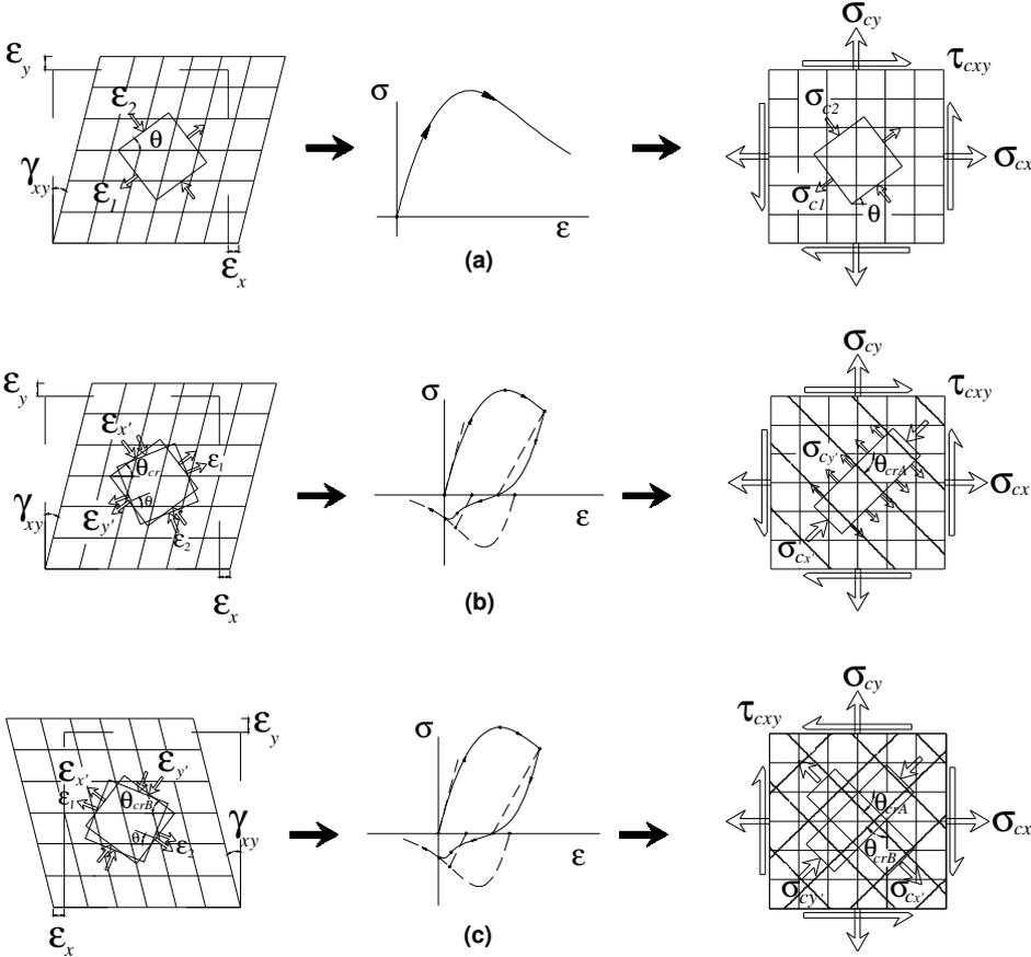
**Figure 1.** Concrete biaxial behavior in the Fixed Strut Angle Model: (a) uncracked behavior, (b) behavior after formation of first crack, (c) behavior after formation of second crack
