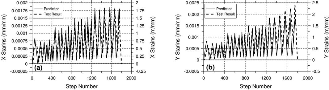
**Figure 5.** Average normal strain histories for Specimen SE9: (a) in x direction, (b) in y direction
