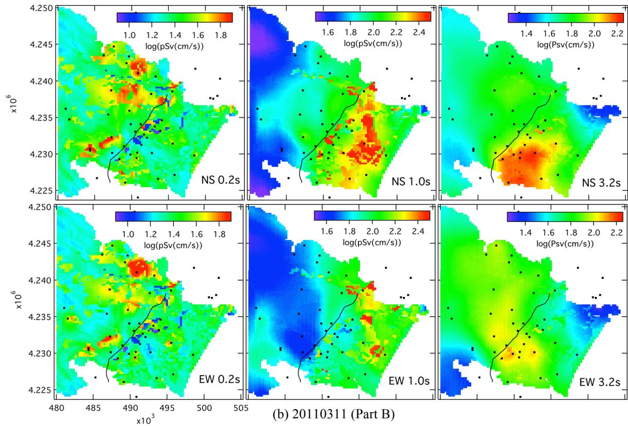
**Figure 8.** Estimated distribution of response spectra at ground surface for the 2011 Tohoku earthquake
