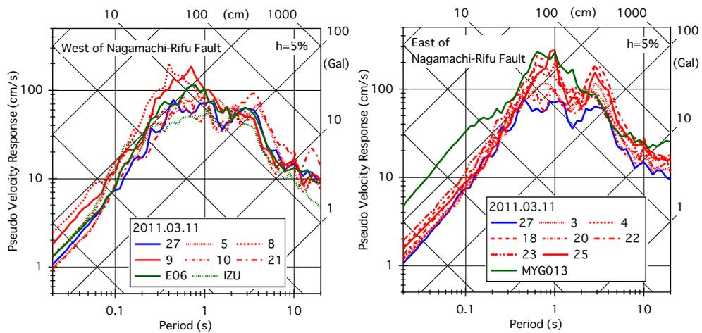
**Figure 4.** Pseudo velocity response spectra of the DCRC records for the 2011 Tohoku earthquake
