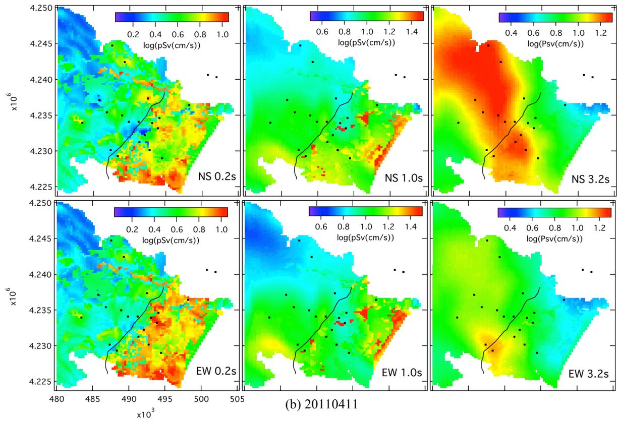
**Figure 9.** Estimated distribution of response spectra for the aftershocks of the 2011 Tohoku earthquake
