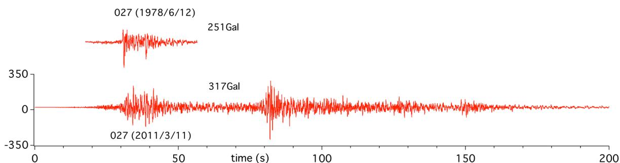
**Figure 5.** Acceleration waveforms at No.27 station for the 1978 Miyagi-oki and 2011 Tohoku earthquakes
