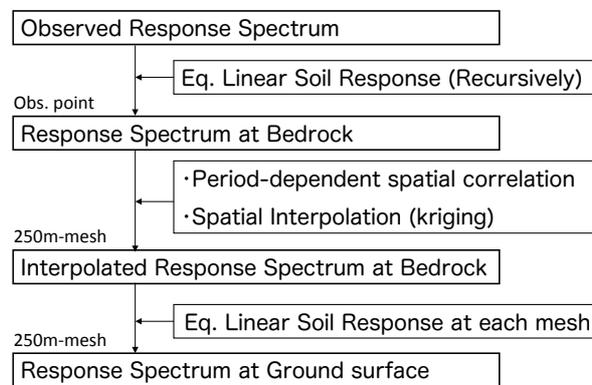
**Figure 7.** Flowchart of estimating distribution of response spectra in Sendai (Ohno and Shibayama, 2010)
