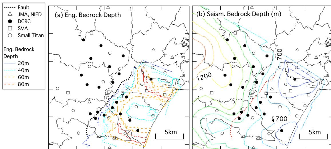
**Figure 2.** Depths of engineering bedrock and seismic bedrock in Sendai (Sendai City, 2002)
