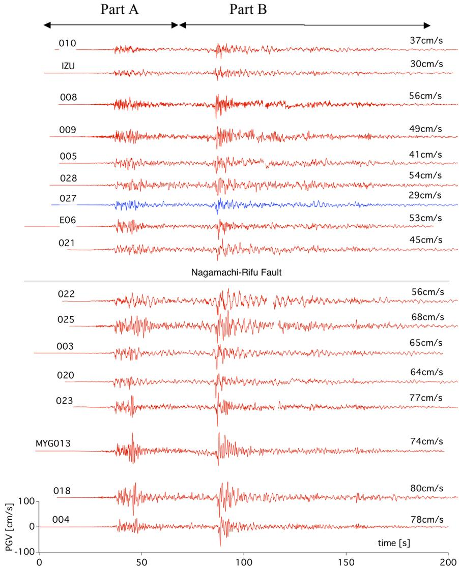
**Figure 3.** Velocity waveforms of the DCRC records for the 2011 Tohoku earthquake
