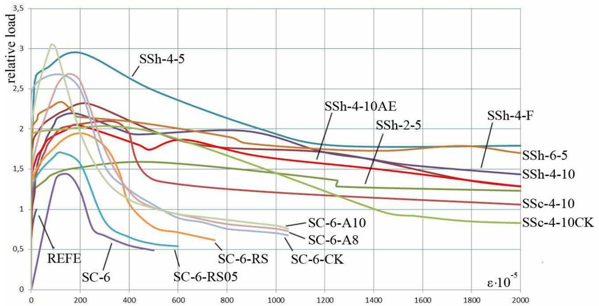
Figure 3. Diagrams of masonry deformation (tension)
