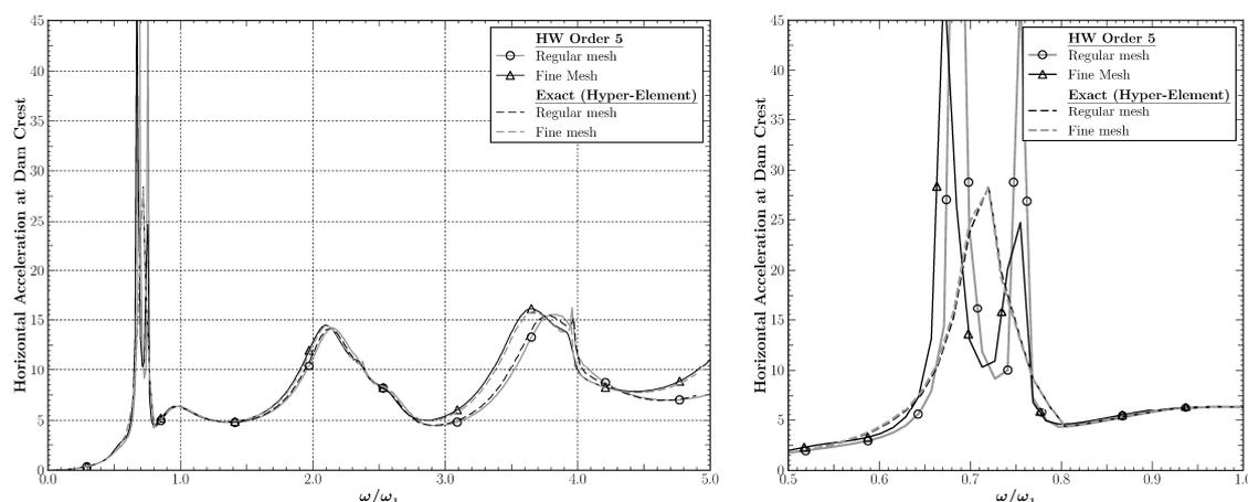
**Figure 5.** Horizontal acceleration at the dam crest due to horizontal excitation for order 5 boundary condition and hyper-element method, by regular and refined meshes ( $L/H = 1.0$  and  $\alpha = 1$ ).
