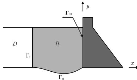
**Figure 1.** Schematic view of a 2D dam-reservoir system.
