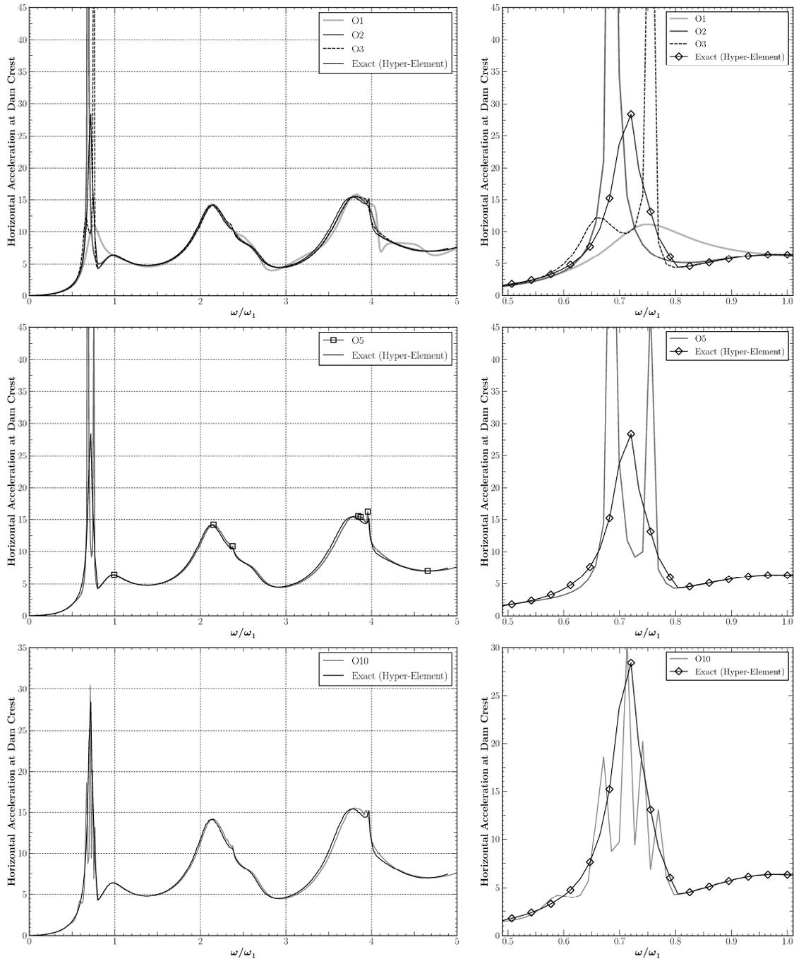
**Figure 4.** Horizontal acceleration at the dam crest due to horizontal excitation for different orders of H-W boundary condition ( $L/H = 1.0$  and  $\alpha = 1$ ).
