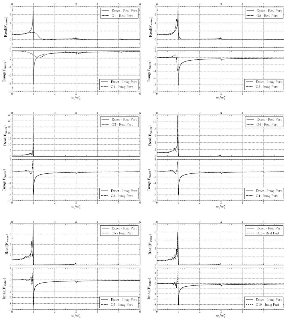
**Figure 6.** Hydrodynamic force ( $F_{water}$ ) on a rigid wall for different orders of H-W boundary condition, due to horizontal ground motion ( $L/H = 1$ ,  $\alpha = 1$ ).
