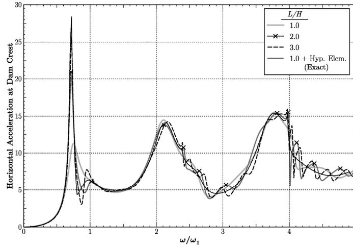
**Figure 3.** Horizontal acceleration at the dam crest due to horizontal excitation for models with different ratios of  $L/H$  and applying Sommerfeld BC on  $\Gamma_1$ .
