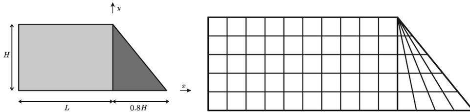
**Figure 2.** (a) Geometry of the model, used in numerical analyses, and (b) the corresponding FE mesh for  $L/H = 2.0$ .
