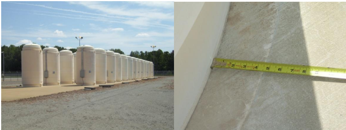
Figure 6. TransNuclear casks at the NANPS (left) and some of the casks were moved as far as 11.4 cm (right).
