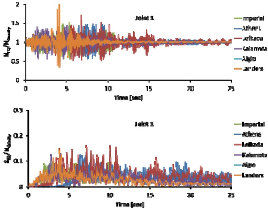
**Figure 11.** Time histories of the normalized normal and shear forces induced at the lower joint 1 of column 1 of the Olympeion for all earthquake motions considered.
