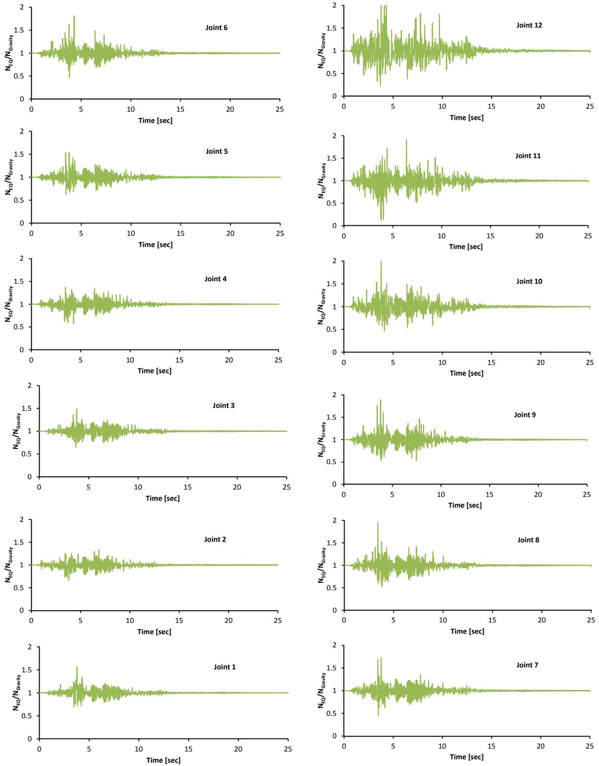
**Figure 9.** Time histories of the normalized normal forces induced at the joints of the column of the Parthenon Pronaos during the Aigio Earthquake.
