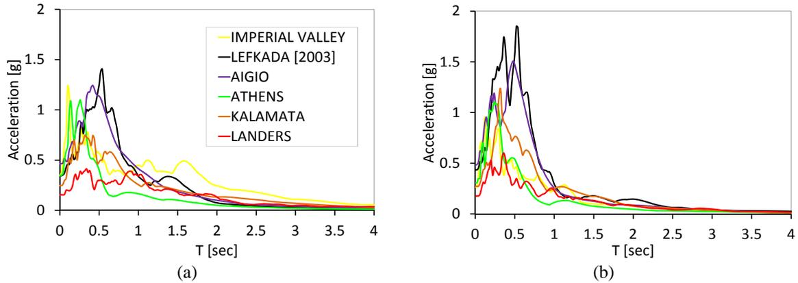
**Figure 6.** Acceleration response spectra for 5% damping of the horizontal components of the base motions that were applied in: (a) the longitudinal direction and (b) the transverse direction of the monuments.
