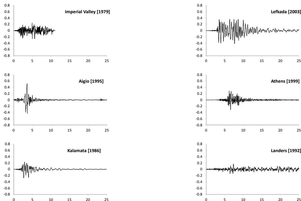
**Figure 5.** Acceleration time histories of the earthquake records applied in the transverse direction of the monuments.
