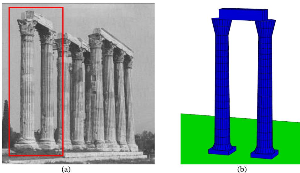
**Figure 3.** (a) SE corner of the Olympieion in Athens. The considered columns are the ones in the red frame; (b) Numerical model used in the analyses.
