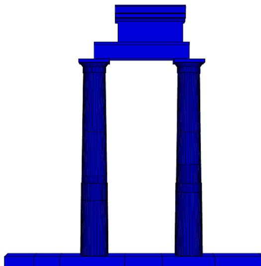
**Figure 1.** Numerical model of the part of the southern Arcade of the Ancient Agora in Kos used in the analyses.
