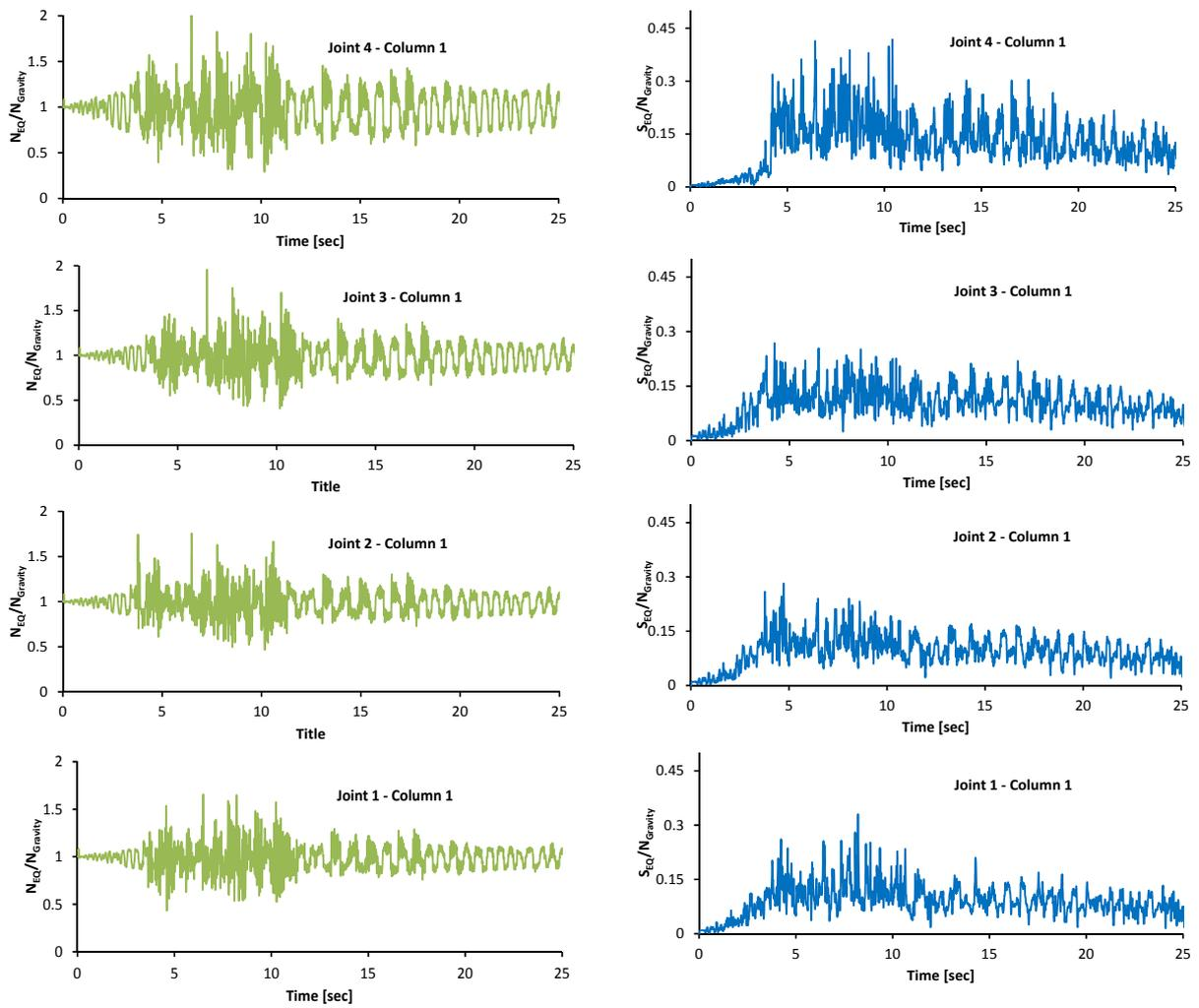
**Figure 7.** Time histories of the normalized normal (left column) and shear (right column) forces induced at the joints of column 1 of the colonnade in Kos during the Lefkada Earthquake.
