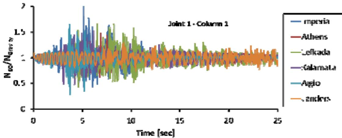
**Figure 8.** Time histories of the normalized normal forces induced at the lower joint 1 of column 1 of the colonnade in Kos for all earthquake motions considered.
