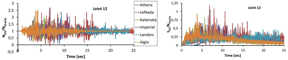
**Figure 10.** Time histories of the normalized normal and shear forces induced at the highest joint 12 of the column of the Parthenon Pronaos for all earthquake motions considered.
