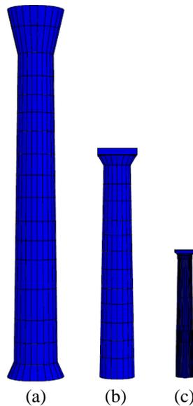
**Figure 4.** Comparison of the size of the columns of the three monuments considered: (a) Olympieion; (b) Pronaos; (c) Kos.
