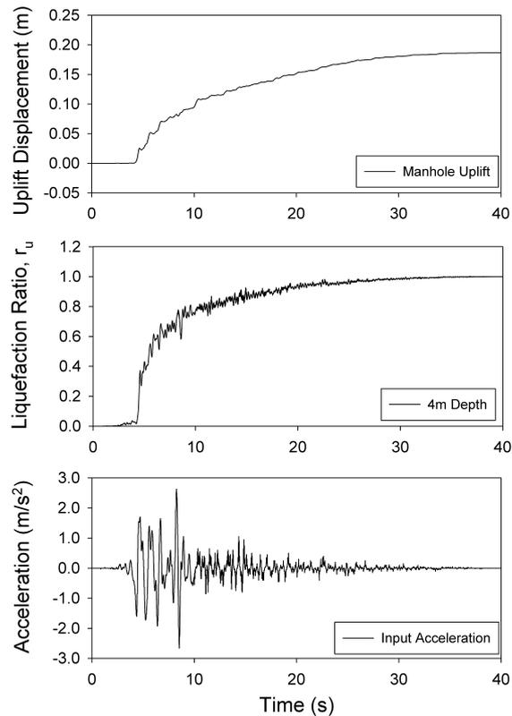
**Figure 6.** Uplift displacement of manhole, base input motion and liquefaction ratio at 4m depth 1.5m away from manhole
