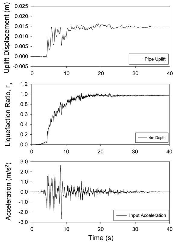
**Figure 8.** Uplift displacement of pipe, base input motion and liquefaction ratio at 4m depth 1.5m away from pipe
