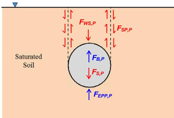
**Figure 3.** Forces acting on a pipe in liquefied soil
