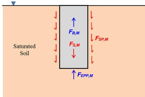
**Figure 4.** Forces acting on a manhole in liquefied soil
