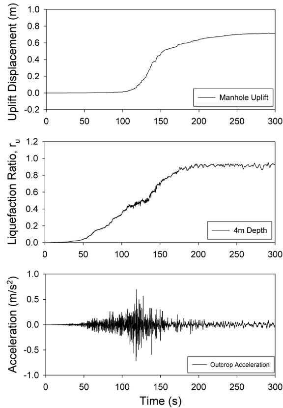
**Figure 9.** Uplift displacement of manhole, base input motion and liquefaction ratio at 4m depth, obtained from analysis representing the Tōhoku earthquake at Urayasu
