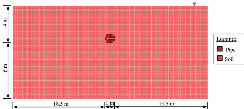
**Figure 7.** Model layout with buried pipe
