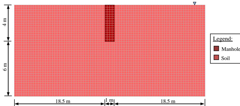
**Figure 5.** Model layout with manhole
