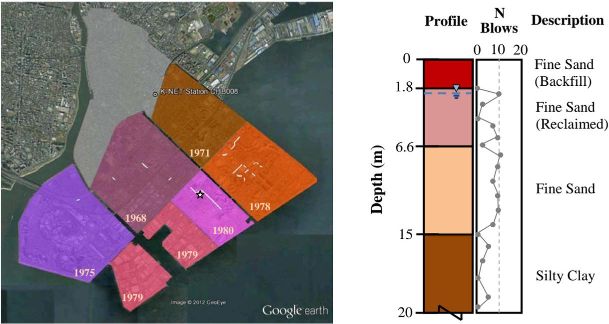
**Figure 2a. (left)** Overview of Urayasu city (shaded) with year of reclamation and locations of significant uplift of manhole (in white lines); from Liquefaction Mitigation Investigation Committee, Chiba Prefecture (2011)
