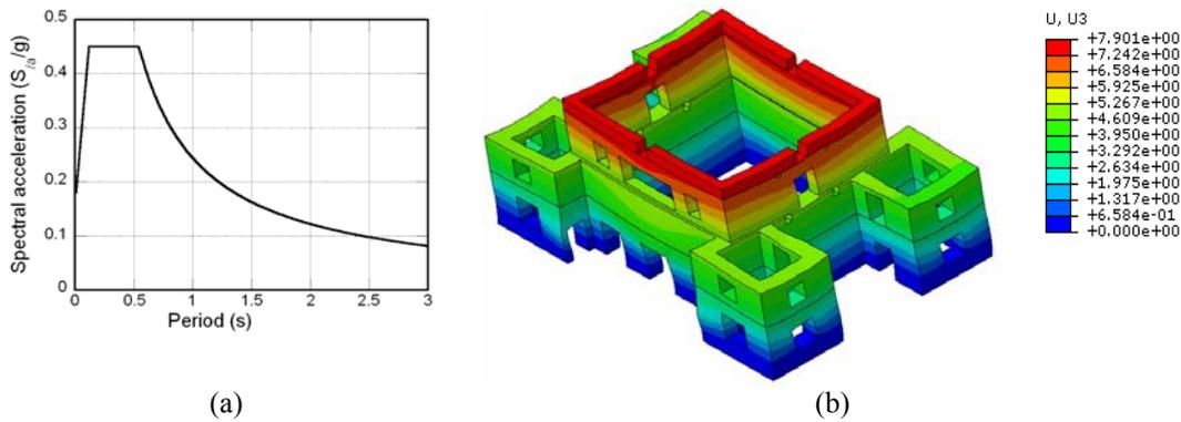
**Figure 5.4.** (a) Response spectrum for zone IV soil type II with 5% damping and (b) Displacement contour for loading in  $y$ -direction as obtained by RSA
