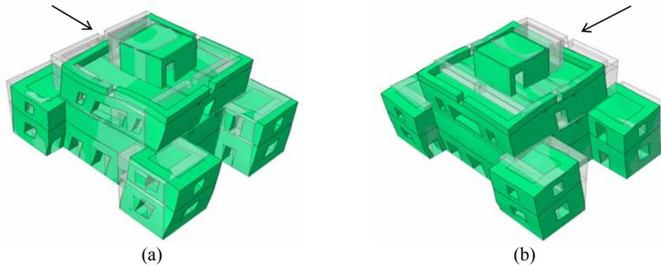
**Figure 5.3.** Mode shapes for natural frequency in (a)  $x$ -direction and (b)  $y$ -direction
