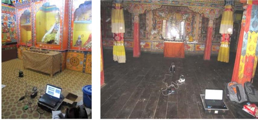
**Figure 4.1.** Experimental setup consisting of seismometer and data acquisition system at Enchey monastery and Labrang monastery.
