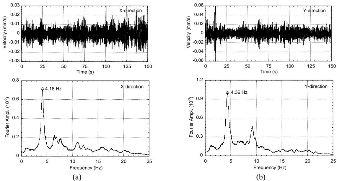
**Figure 4.2.** Recorded time-history and Fourier spectrums at the top floor of Enchey monastery (a) in  $x$ -direction parallel (b)  $y$ -direction perpendicular to the main entrance
