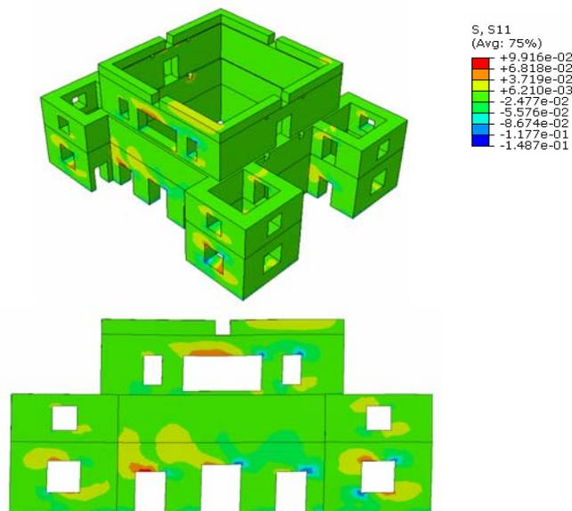
**Figure 5.5.** Areas identified with critical stresses ( $x$ -direction)
