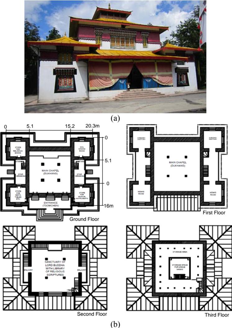
**Figure 5.1.** (a) A view of the main temple at Enchey Monastery and (b) Floor plans at different floor level (Gurung, 2008)
