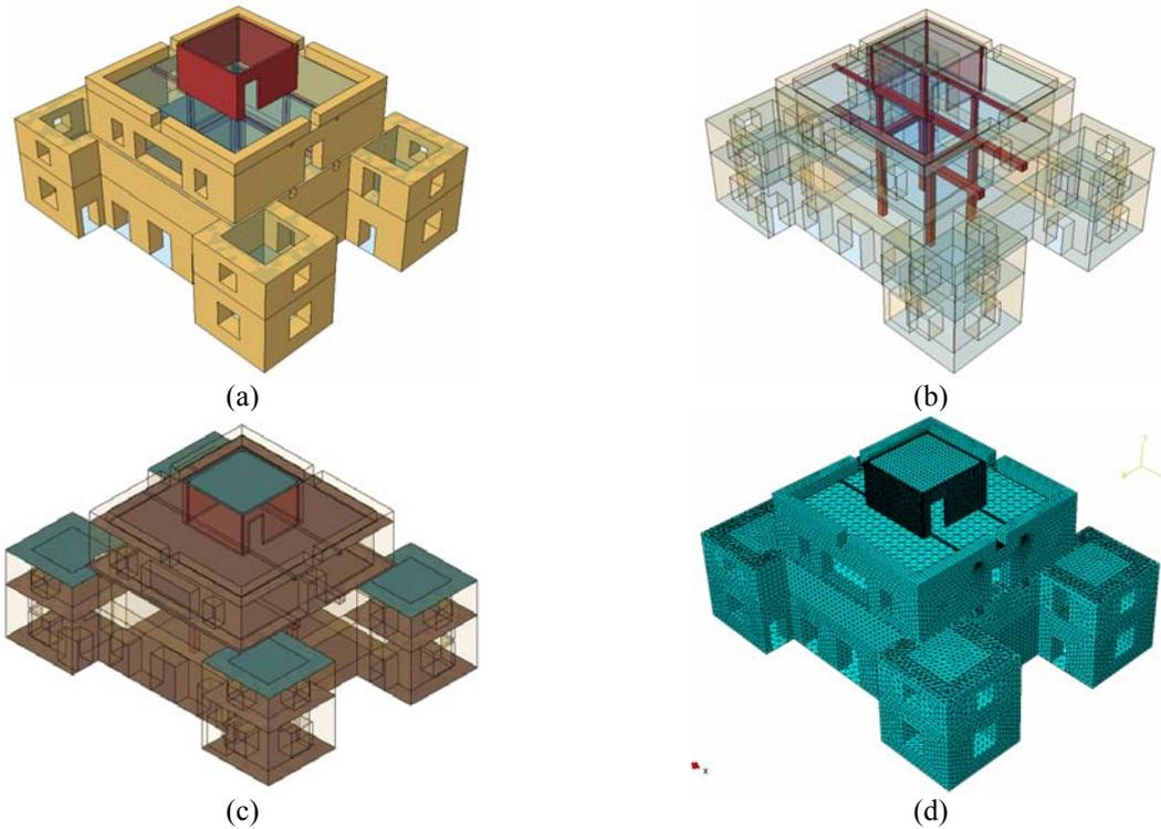
**Figure 5.2.** View of model showing (a) Exterior masonry walls and small wooden cabin (b) Frame system of the structure comprising of wooden beams and columns (c) Roof and floor diaphragms modeled as flat slabs using solid shell elements and (d) Discretization of model using tetrahedral and triangular elements.
