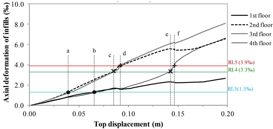
**Figure 9.** Local inelastic responses of the infill panels of the fully infilled 6-story frame structure with equal interstory heights.
