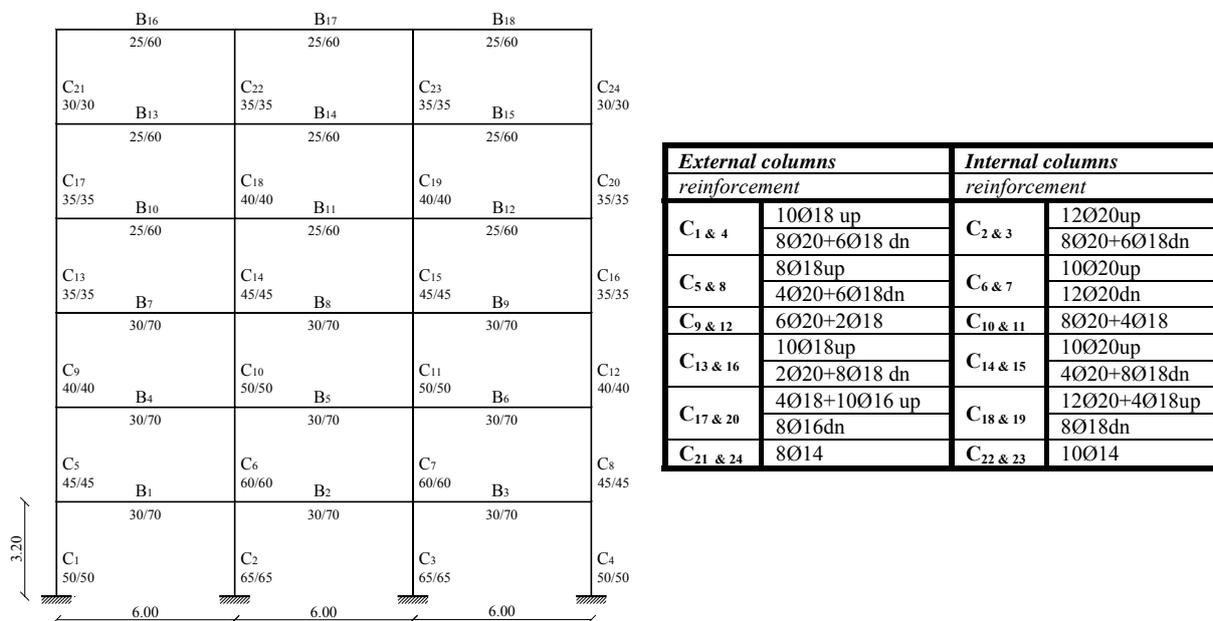
Figure 1. Structural system and column reinforcements of 6-storey RC frame.
