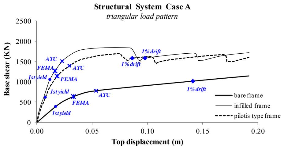
**Figure 3.** Capacity curves of the 6-story frame structures with equal interstorey heights.
