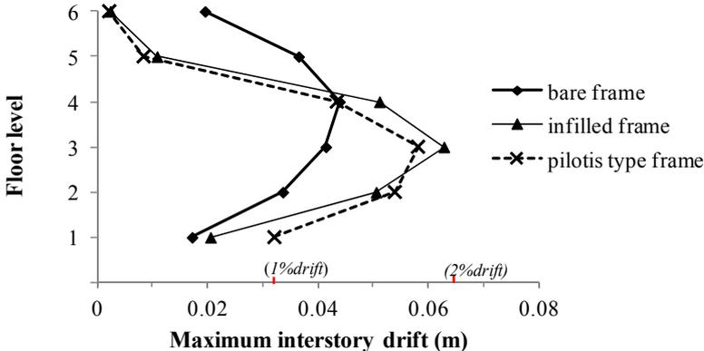
**Figure 5.** Maximum interstory drifts of the 6-story frame structures with equal interstory heights (Case A) at top drift equal to  $1\%h_{str}$ .
