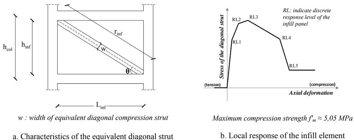
**Figure 2.** Simulation of the infill panel based on the diagonal strut model
