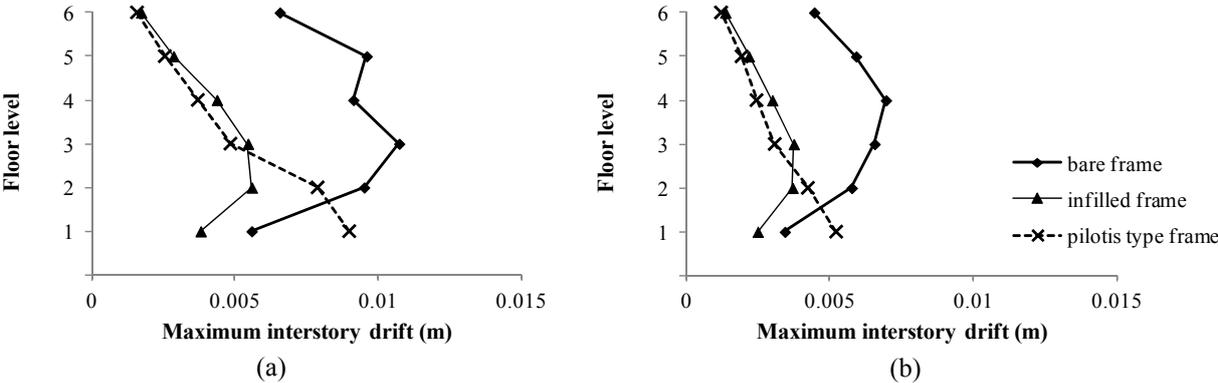
**Figure 6.** Maximum interstory drifts of the 6-story frame structures with equal interstory heights (Case A): a) at performance points to ATC40 and b) at target displacement to FEMA356.
