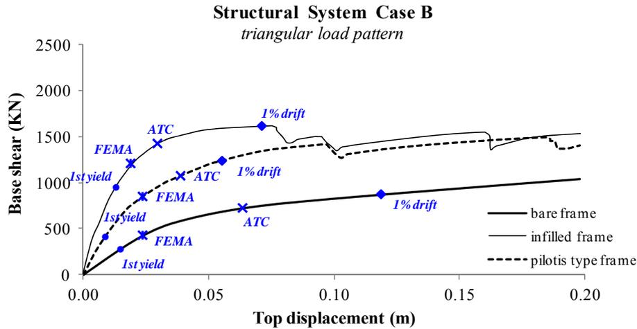
**Figure 4.** Capacity curves of the 6-story frame structures with the height at the base to be greater than the other equal interstory heights (Case B).
